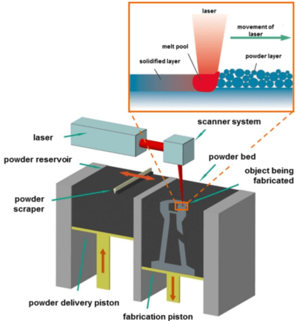
*Figure 3. 1: Direct Metal Laser Sintering (DMLS)[21]*
