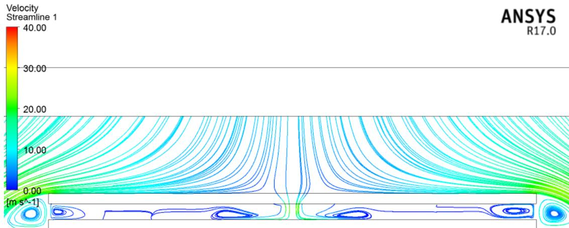
Figure 8.4: Flow streamlines for 1 mm air gap
