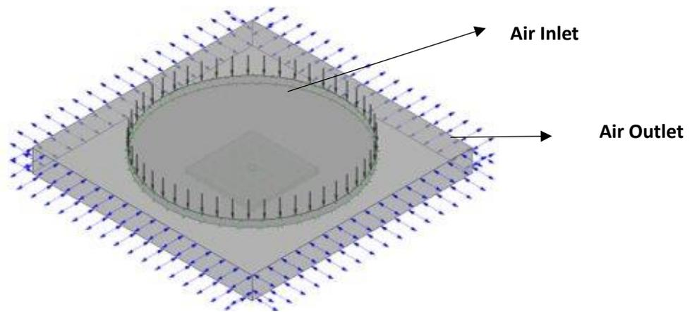
*Figure 8. 1: Boundary conditions for the environment*
