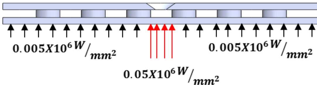
*Figure 8. 2: Boundary conditions to the heat spreader*
