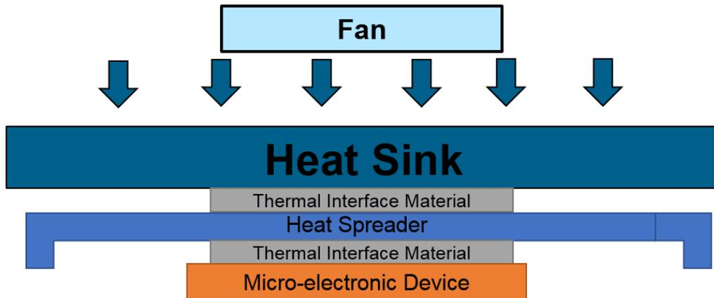
*Figure 2. 1: Conventional air-cooled thermal management system*
