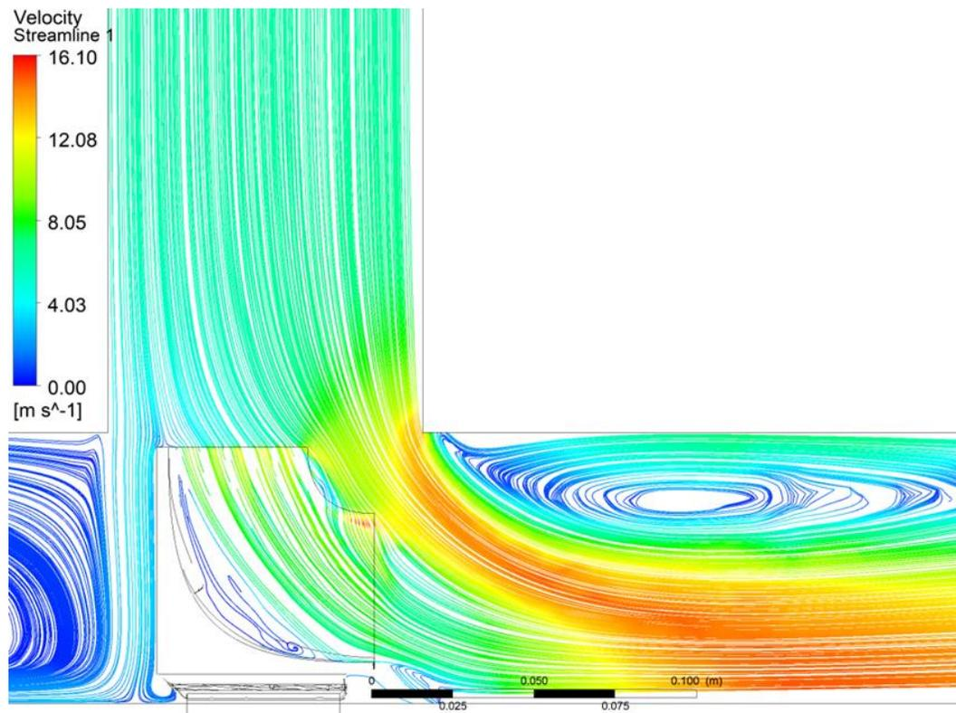
Figure 5. 3: Using laminar fluid flow model
