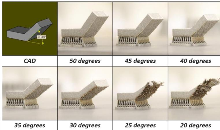
Figure 3. 2: Effects of different feature angles[23]
