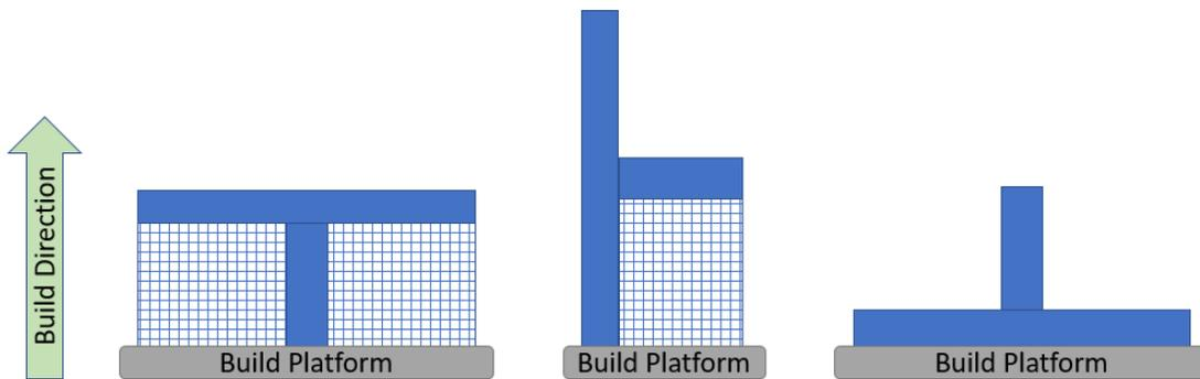
Figure 3. 3: Support required for different orientation of the same part
