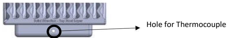
*Figure 6. 2: Thermocouple hole*
