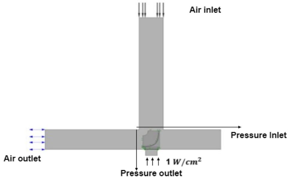
Figure 5. 2: Analysis setup with the boundary conditions
