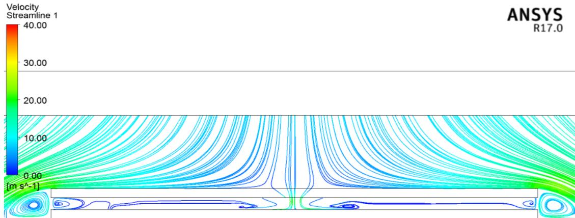
Figure 8.5: Flow streamlines for 0.8 mm airgap
