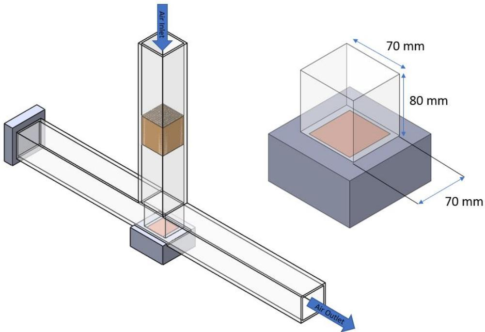
*Figure 6. 1: Experimental setup assumed from the guidelines data*
