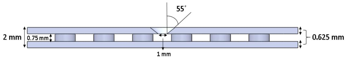
Figure 7. 2: Heat spreader dimensions at the cross section
