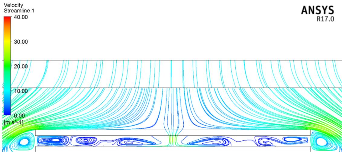
Figure 8.3: Flow streamline for 1.2 mm air gap
