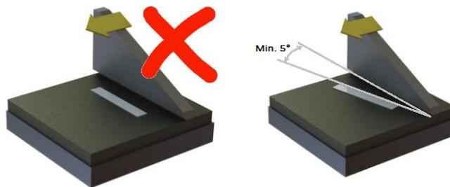
Figure 3. 4: Orientation of the part with the raster[24]
