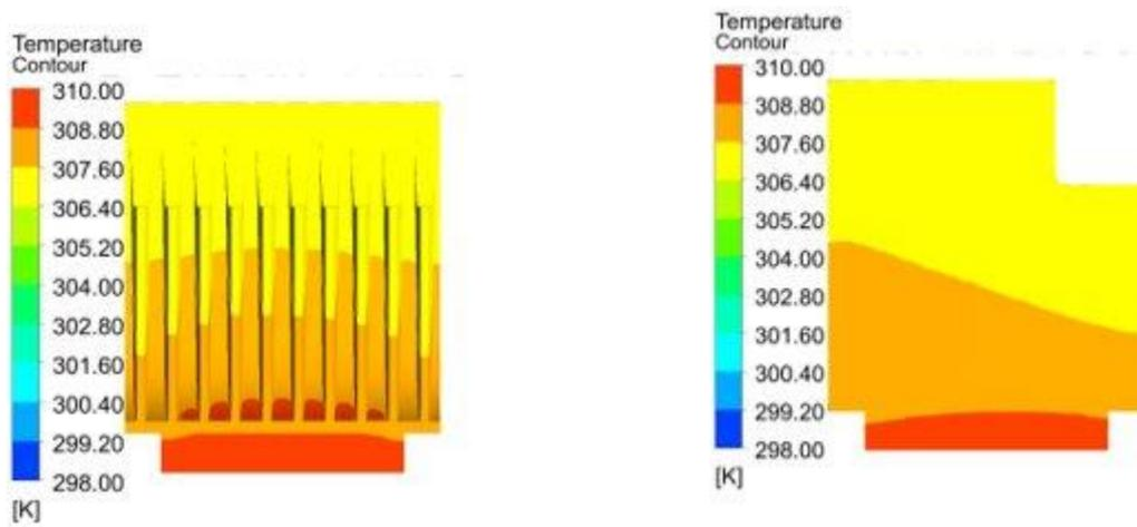
Figure 5. 6: Thermal analysis contour for conventional heat sink
