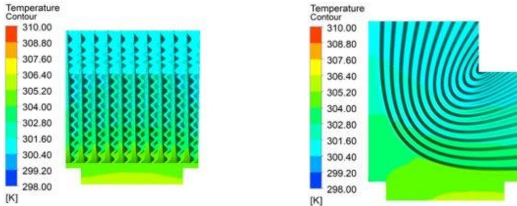
*Figure 5. 5: Thermal analysis contour for the heat sink*
