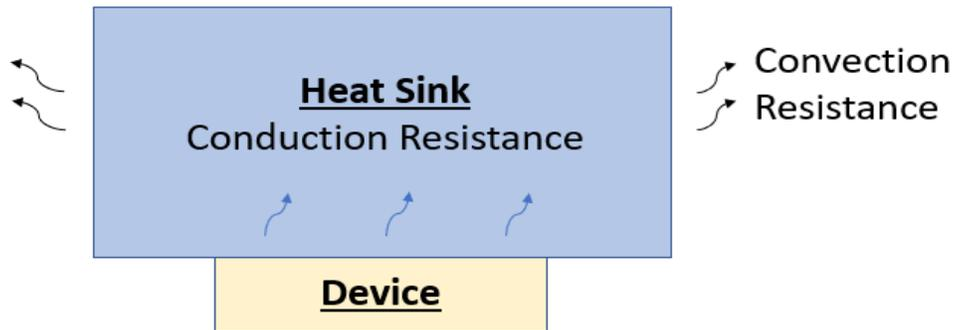
Figure 2. 2: Conduction and convective resistance
