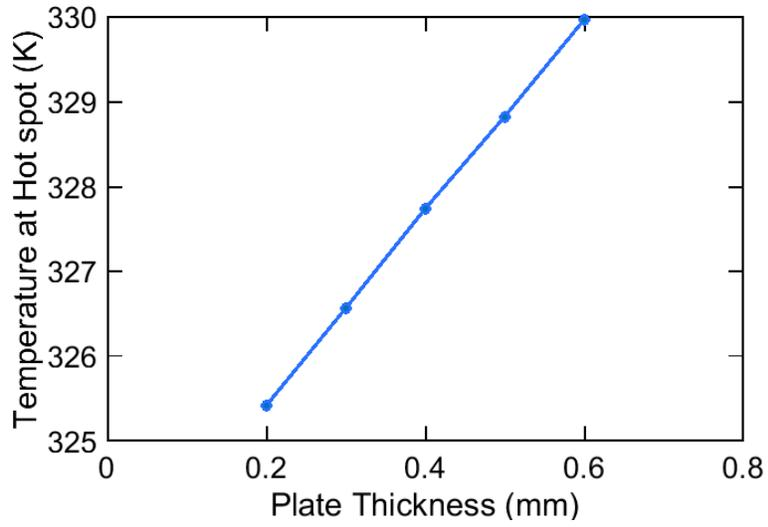
Figure 8. 8: Temperature at hot spot by varying plate thickness with respect to air gap
