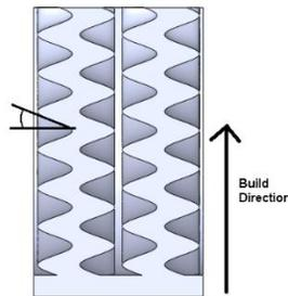
*Figure 4. 5: Model sink for wavelength analysis*
