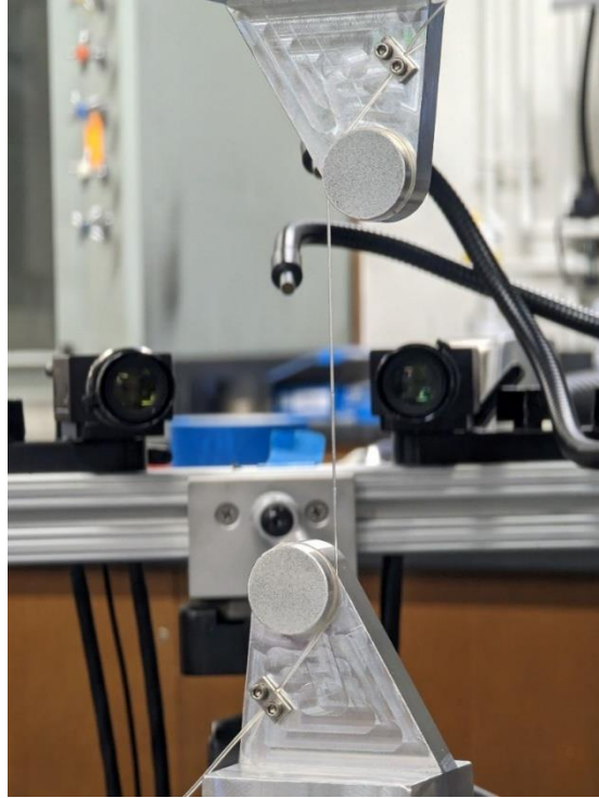
Fig 15: The fiber testing setup designed by the Advanced Materials and Structures Laboratory at UTA.
