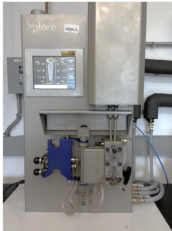
Fig 11: Xplore MC-5 micro compounder
