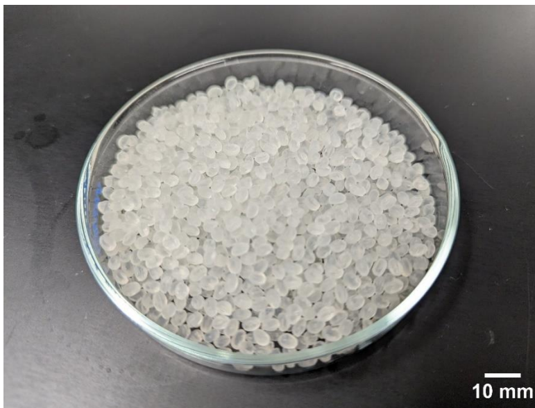
Fig 3: PEBAX® MV 1074 is available to us in the form of natural-colored granules.
