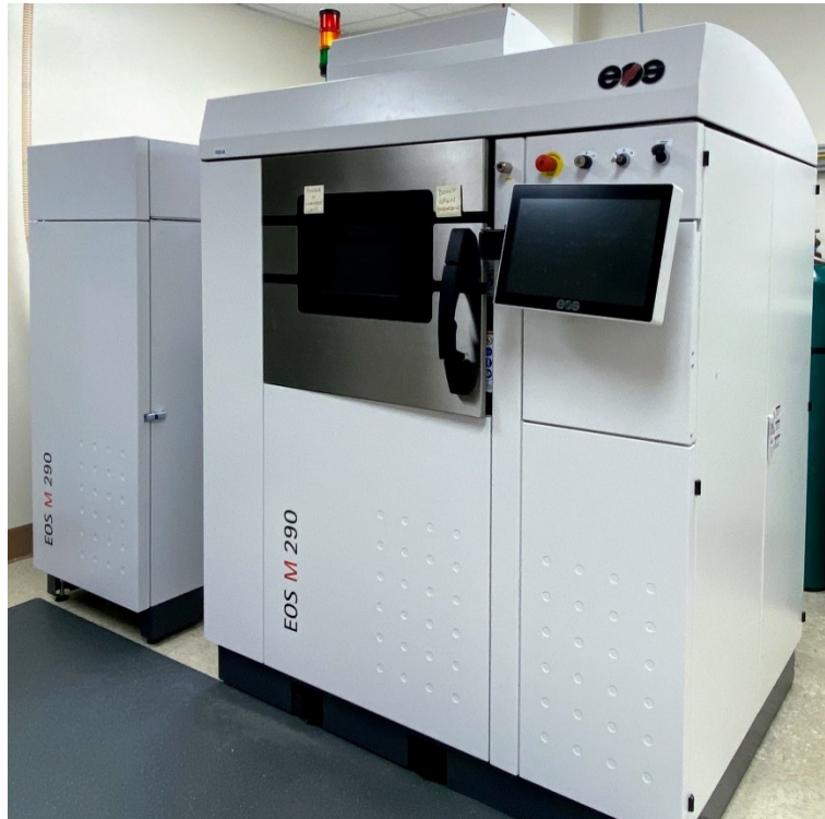
Figure 20. EOS M290 metal 3D printer with a fiber 400 W laser.
