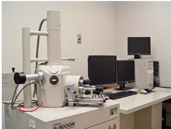
Figure 24. Hitachi S-3000N Scanning Electron Microscope.
