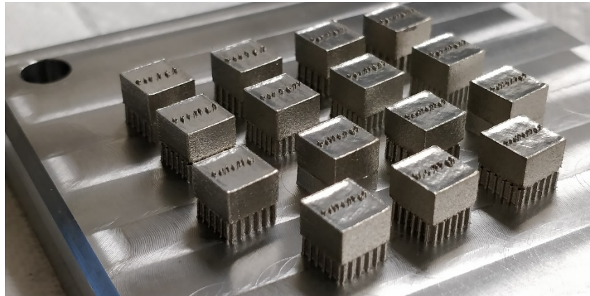
Figure 27. SLM IN718 samples with different support structures fabricated on a stainless-steel building plate.
