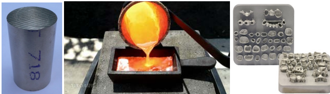
Figure 10. Super-alloy material in a wrought form (left), casting, and powder (middle) and AM (right)[109].
