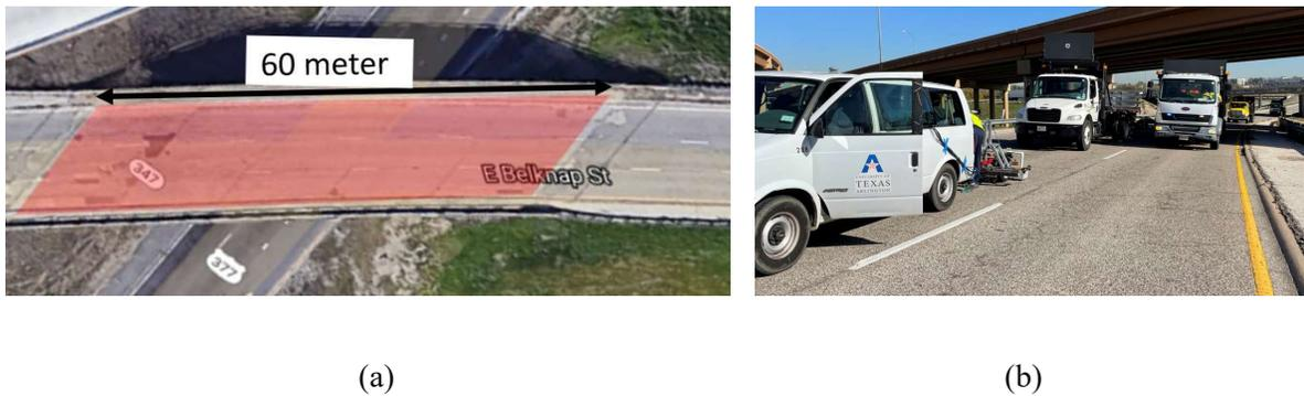
**Figure 4.2.** Field testing photo - (a) scanned area of the bridge, and (b) system and safety control.
