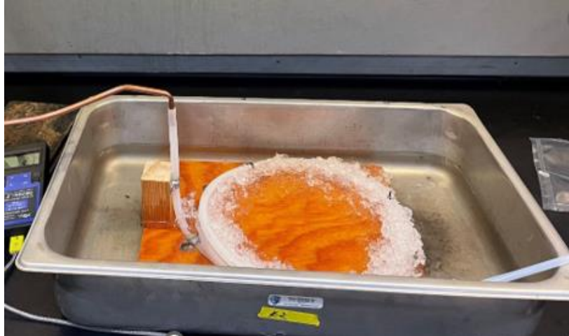
Figure 3.10: Cold trap for the outlet gas
