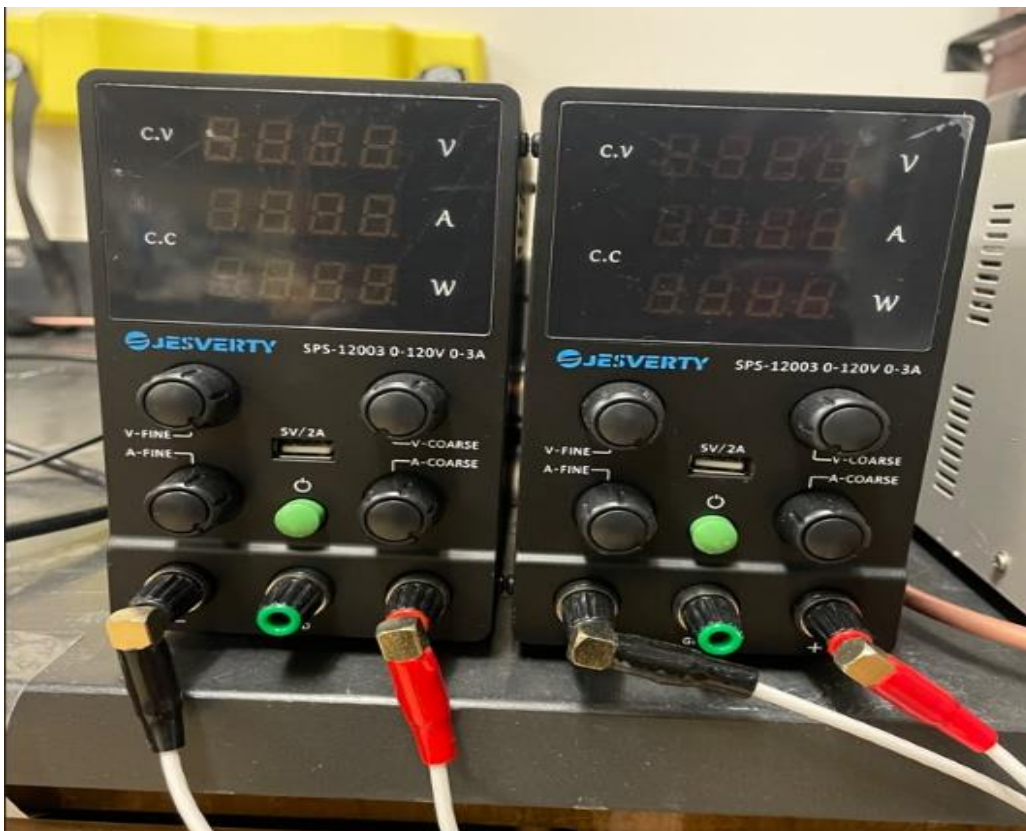
Figure 3.5: DC power supplies in parallel mode (JESVERTY SPS-12003)
