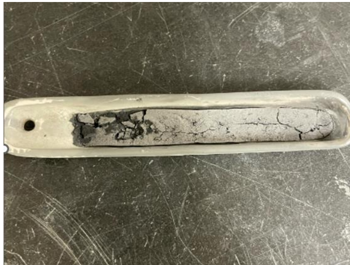
Figure 3.15: Catalyst after heat treatment
