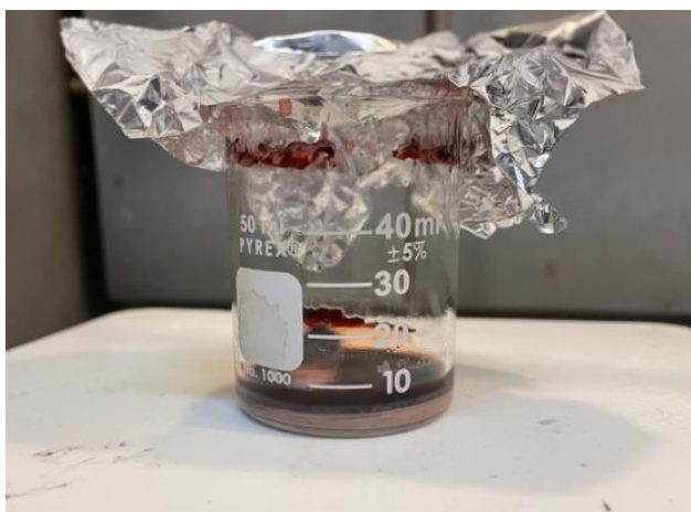
Figure 3.12: Catalyst preparation: stirring and heating.
