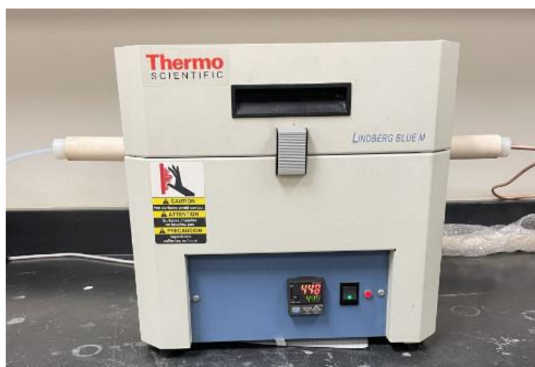
Figure 3.14: Tube furnace: Heat treatment of the catalyst
