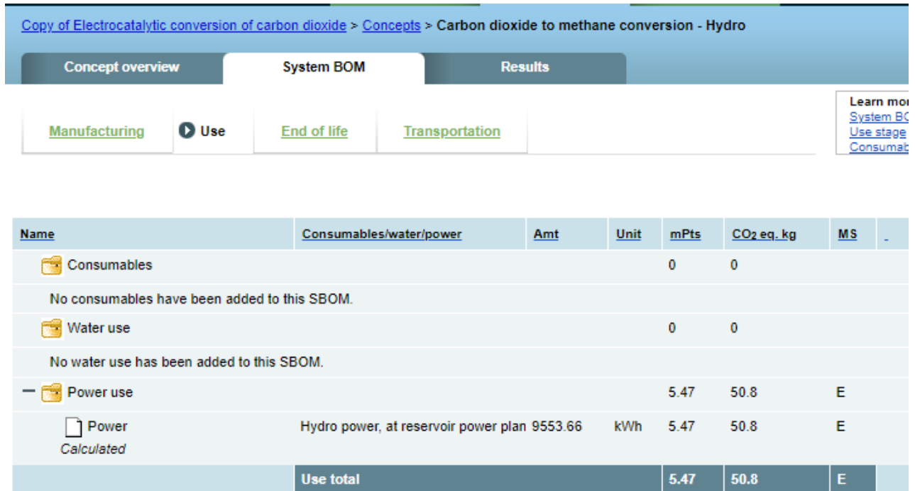
Figure 3.23: Inputs for the use phase of the environmental LCA for the lab-scale Waseda process
