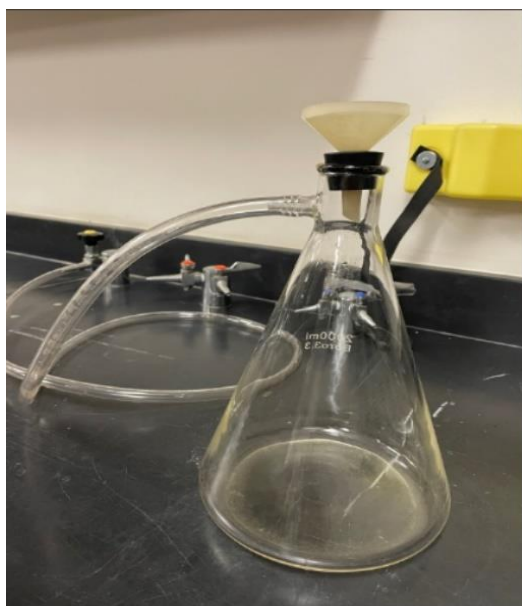
Figure 3.16: Set up of vacuo.
