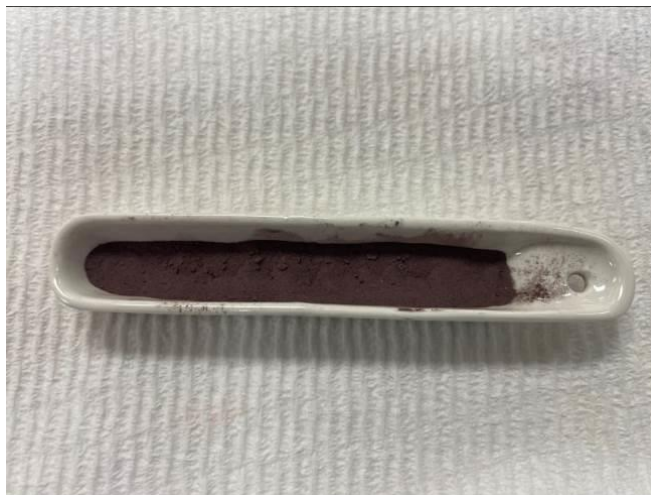
Figure 3.13: Dried catalyst ready for heat treatment
