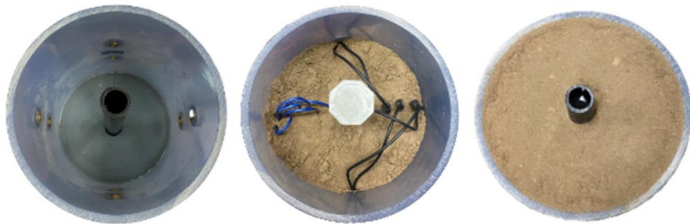
Fig. 5-6. Top view of the soil column at different stages of compaction.
