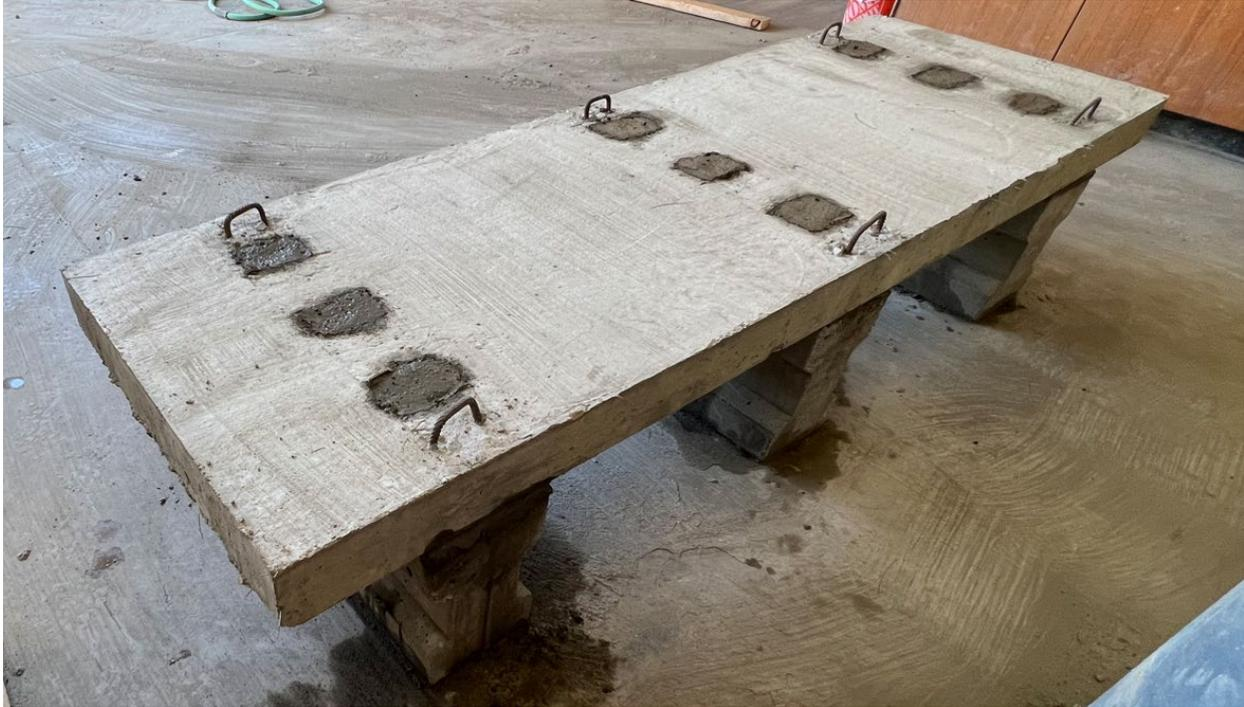
Figure 4 - 9 Precast Deck and Girders After Grouting
