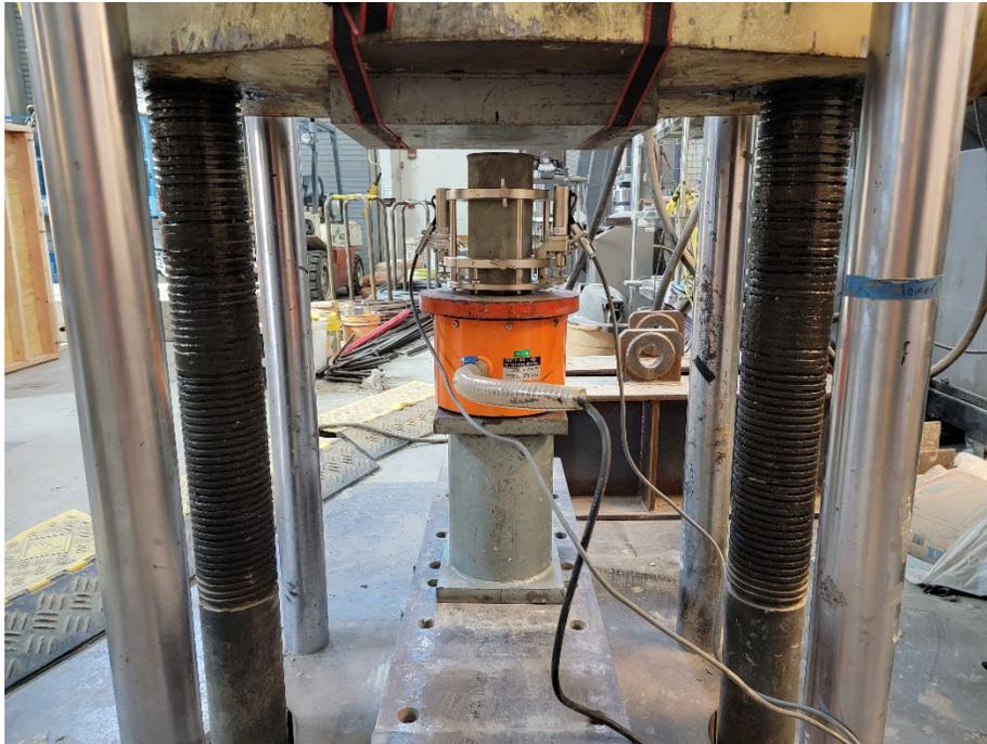
Figure 3 - 25 Modulus of Elasticity Test Machine
