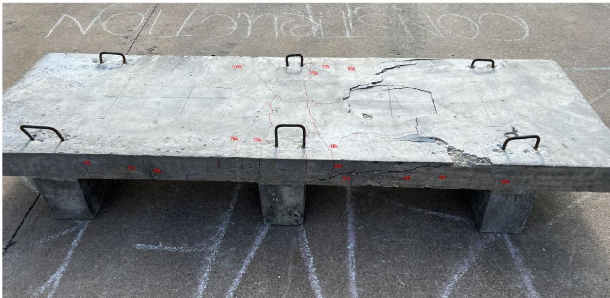
Figure 6 - 5 RC Concrete Deck Specimen
