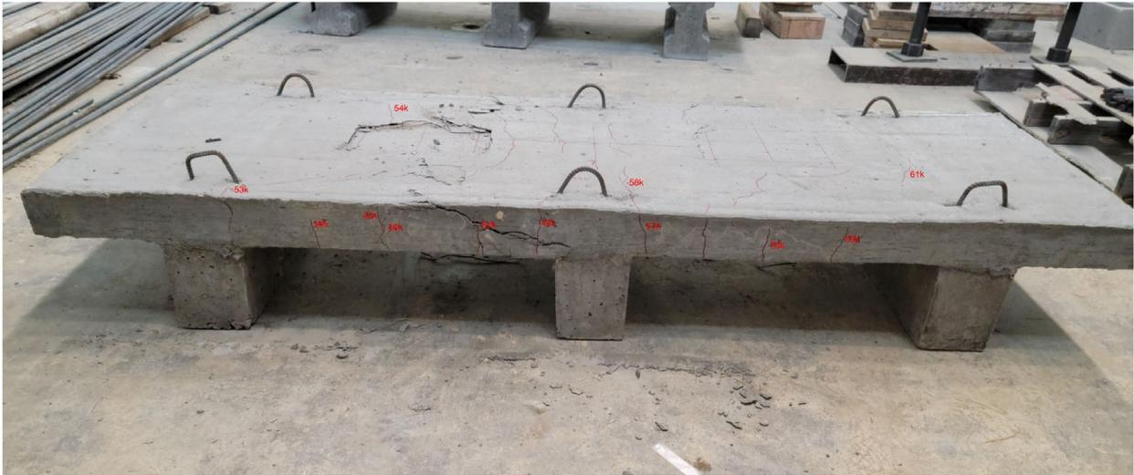
Figure 7 - 5 GFRP Concrete Deck Specimen
