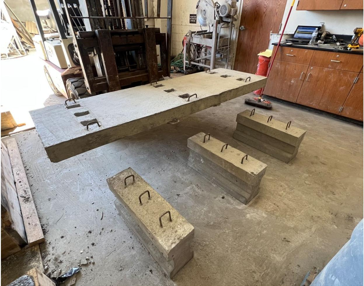
Figure 4 - 8 Precast Deck and Girders before Grouting
