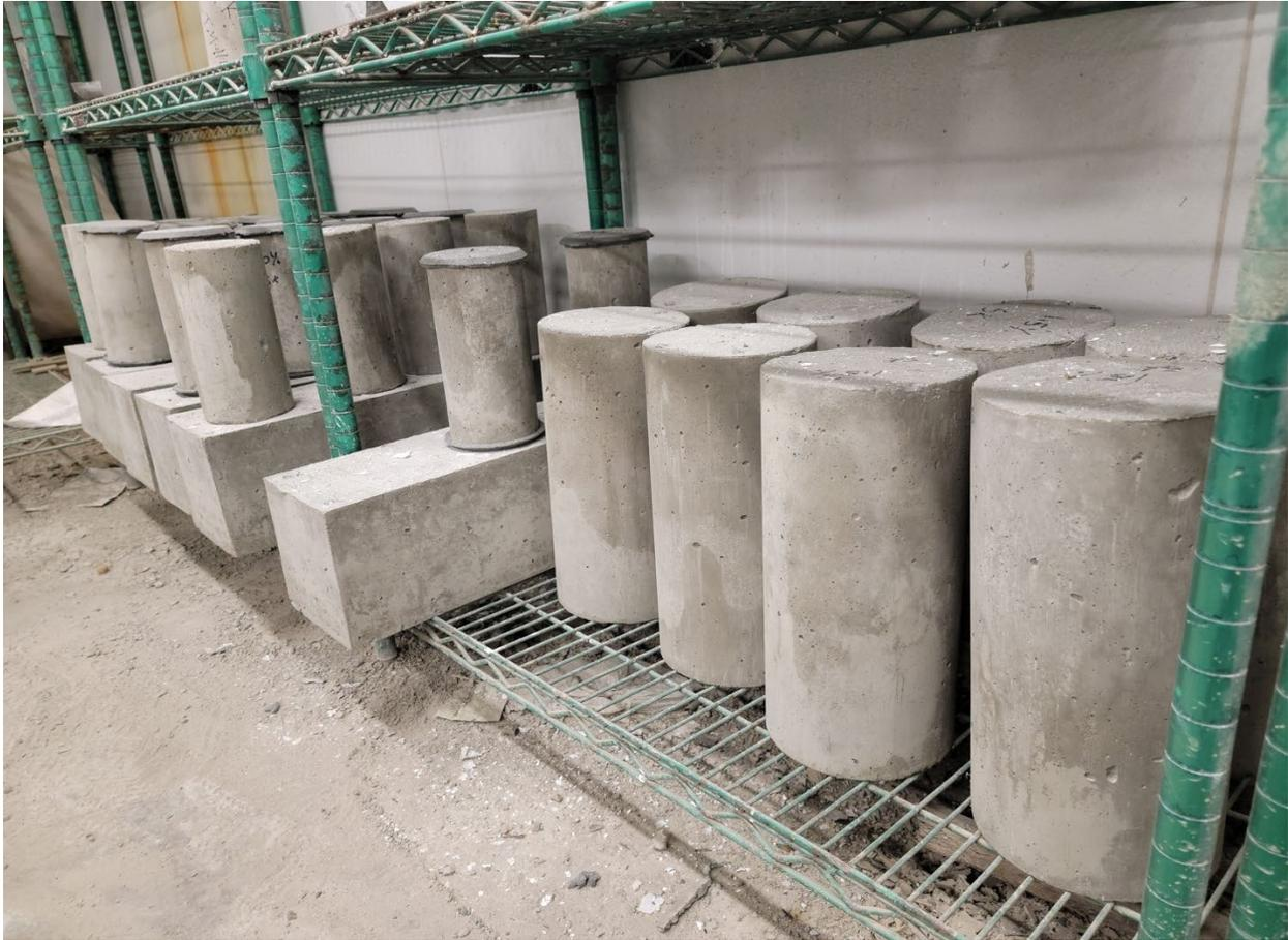
Figure 3 - 6 Concrete Standard Specimens in The Curing Room
