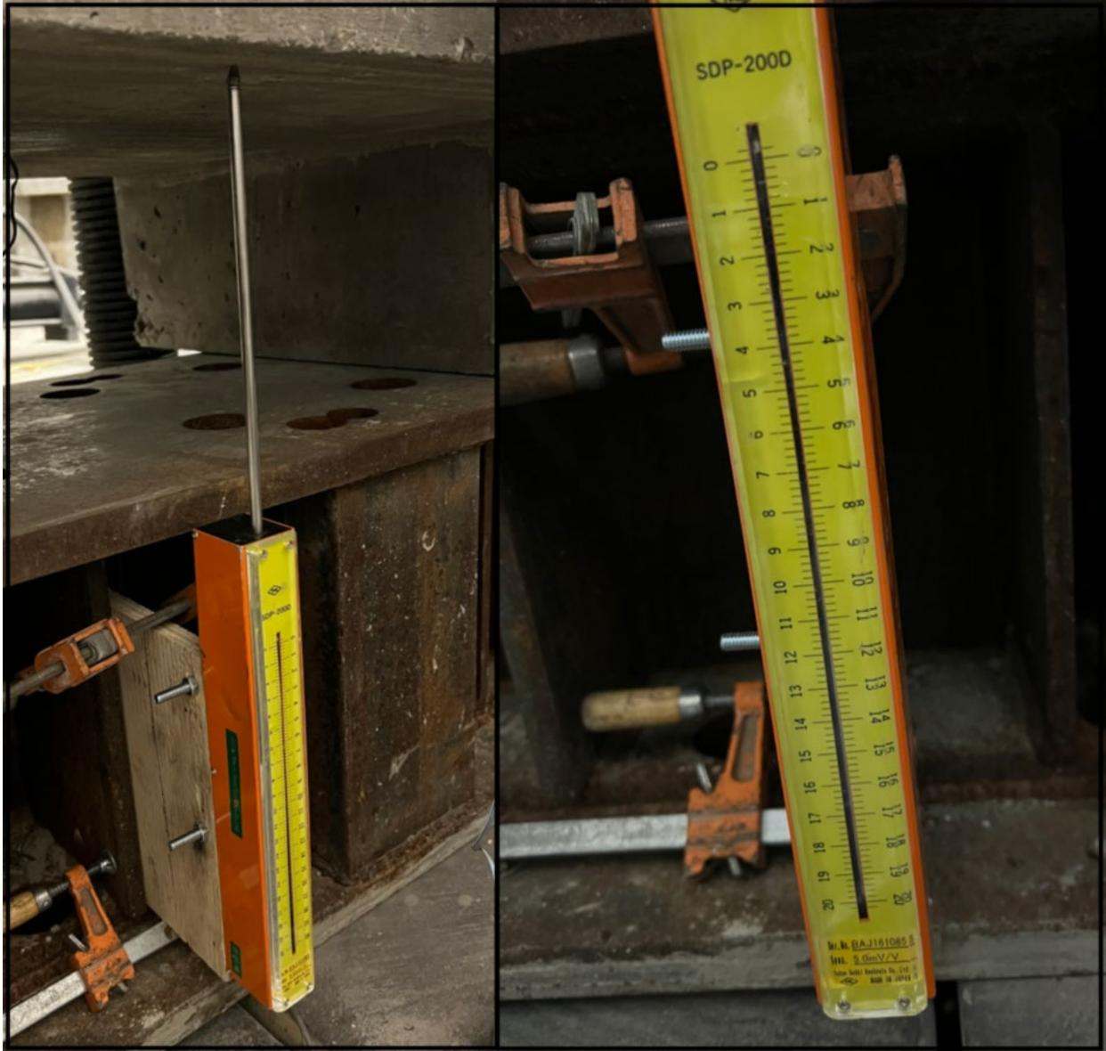
Figure 4 - 19 Linear Variable Differential Transformer Sensor
