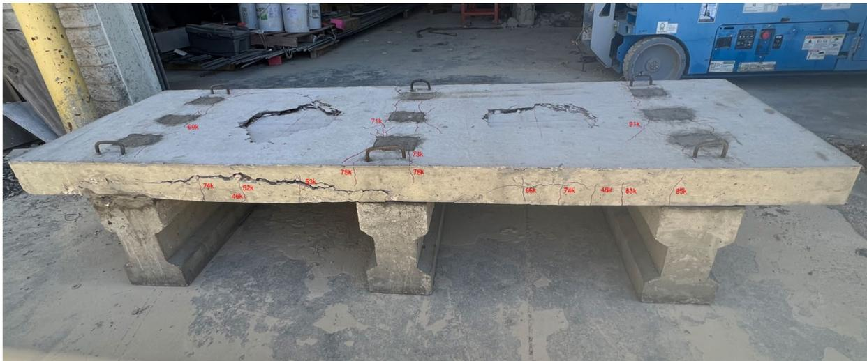
Figure 6 - 15 SFRC-PC Concrete Deck Specimen
