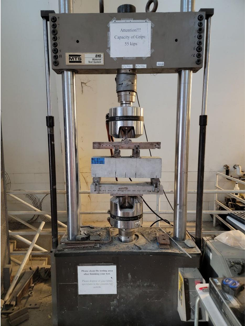
Figure 3 - 19 Flexure Test Machine
