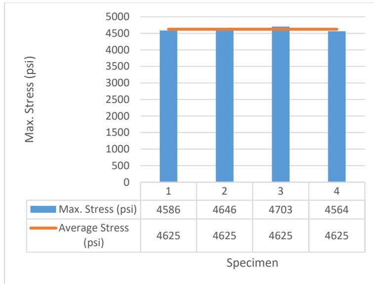
Figure 3 - 12 Ultimate Compressive Strength Test Results of SFRC Concrete
