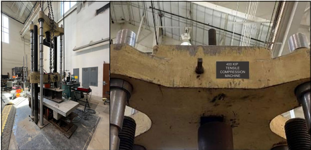
Figure 4 - 15 400 Kips MTS Testing Machine
