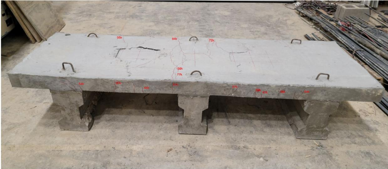
Figure 7 - 10 SFRC-GFRP-CIP Concrete Deck Specimen
