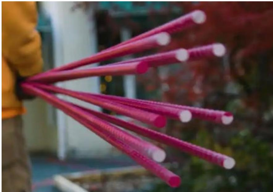
Figure 3 - 5 Glass Fiber Reinforced Polymer Bars (GFRP)
