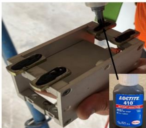
(e) Applying Loctite 410 on steel plate
