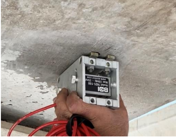
(g) Holding tiltmeter for 10-15 seconds
