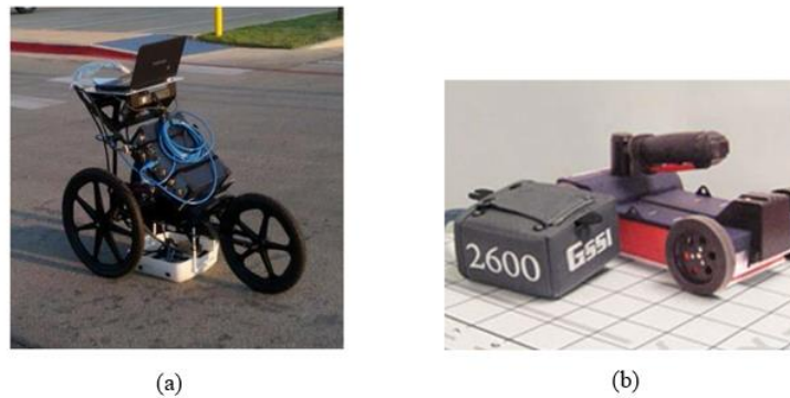
Figure 4-15 Ground penetrating radar (GPR): (a) Cart-mounted GPR; (b) 2.6 GHz antenna
