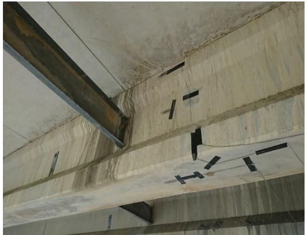
Figure 4-5 Instrumentation plan for load testing: (a) EB bridge; and (b) WB bridge
