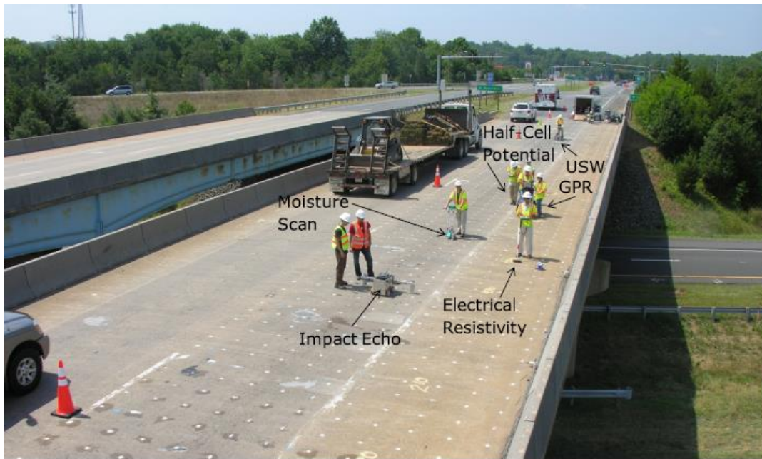
Figure 2-15: NDE technologies during data collection (Gucunski et al. 2016)
