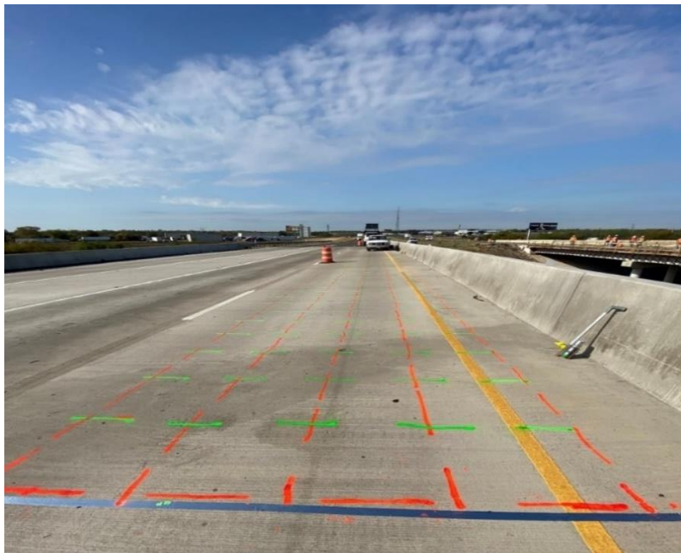
Figure 4-19: GPR and IE scanning grids
