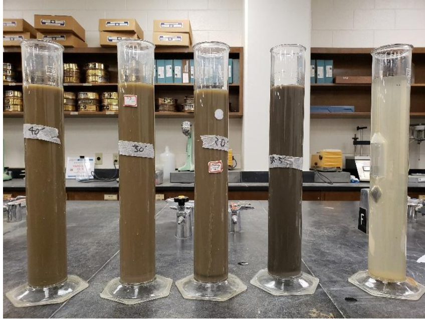
Figure 3.8 Particle size distribution testing using the hydrometer procedure
