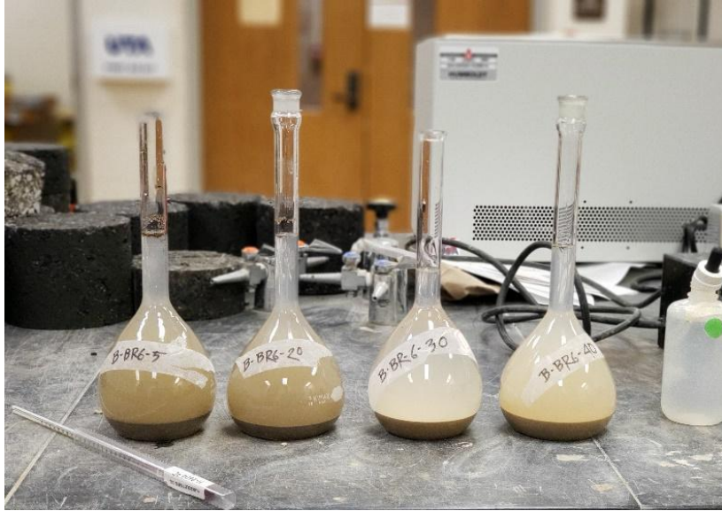
Figure 3.5 Specific gravity testing of soil
