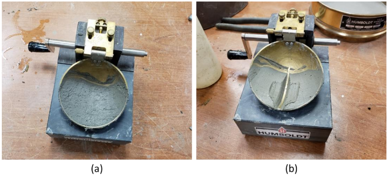
Figure 3.6 Liquid limit testing: (a) the soil is flattened in the device cup, and (b) a groove was made at the center
