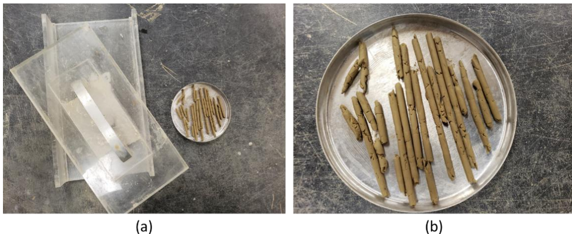
Figure 3.7 Plastic limit testing (a) Rolling device and (b) cracked and broken threads of 3 mm
