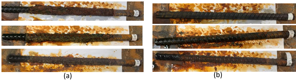
Figure 5.15. AC-T3 rebar with (a) rust particles attached to it, and (b) the rebar after the rust particles were cleaned.
