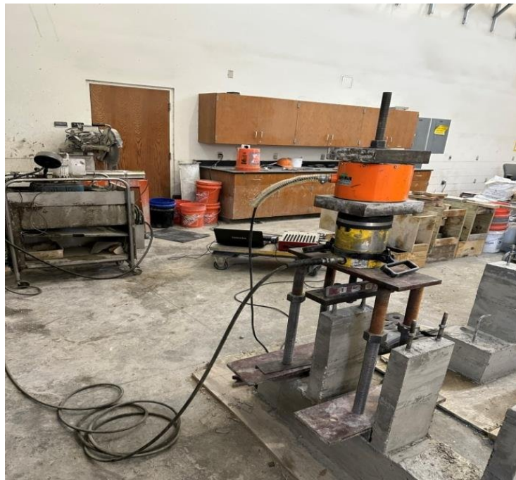
Figure 3.37 Anchor Group Pullout Test Set-Up (Lab)
