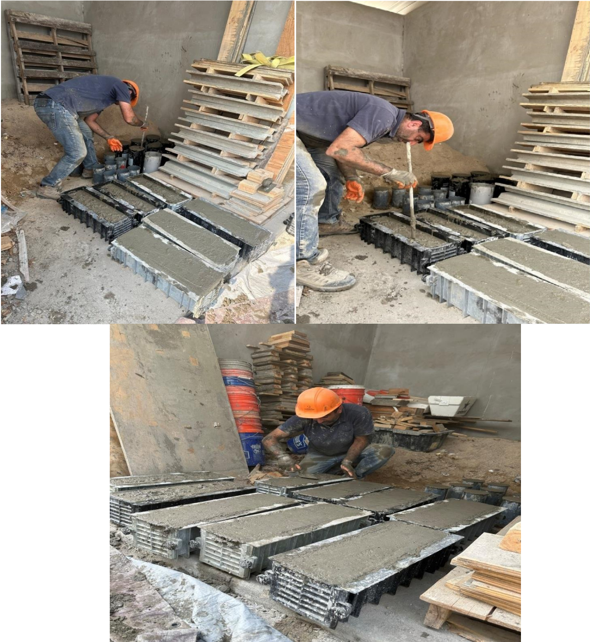
Figure 3.17 Cylindrical and beam specimens
