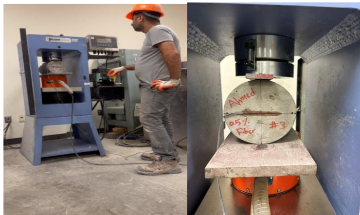
Figure 3.24 Split Tensile Test Set-Up
