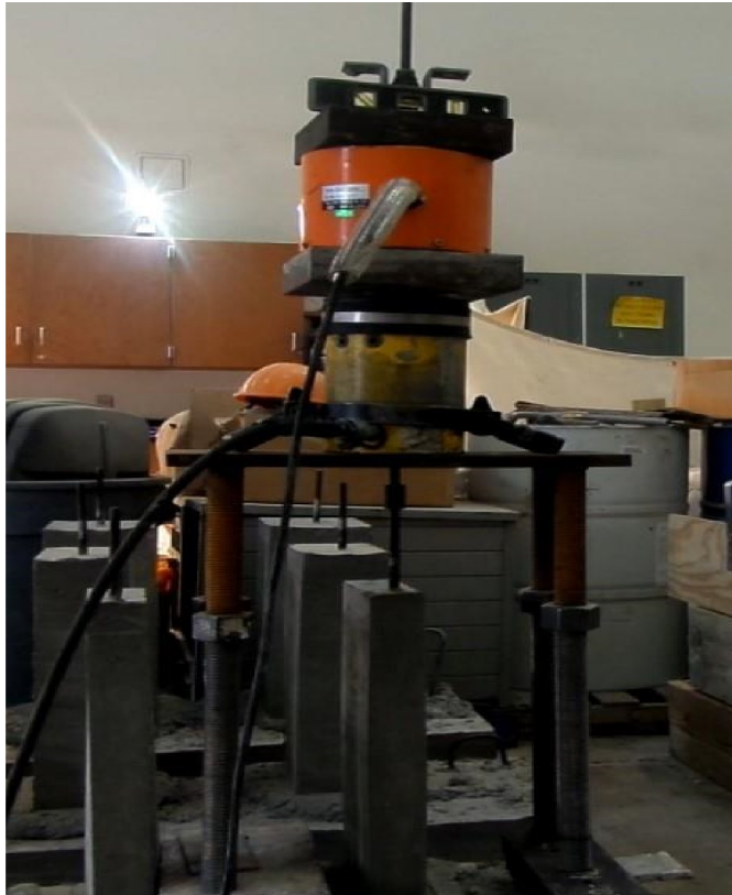
Figure 3.30 Single Anchor Pullout Test Set-Up (Lab)
