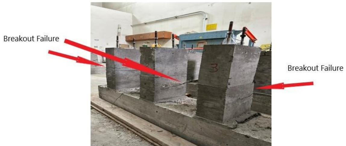
Figure 3.42 Concrete Breakout Failures (1.0% SFRC)
