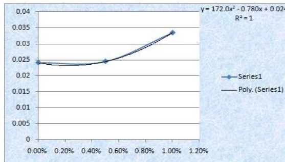
Figure 4.20 Modification Factor (Z) vs. SFRC (%) at (1.0hef)
