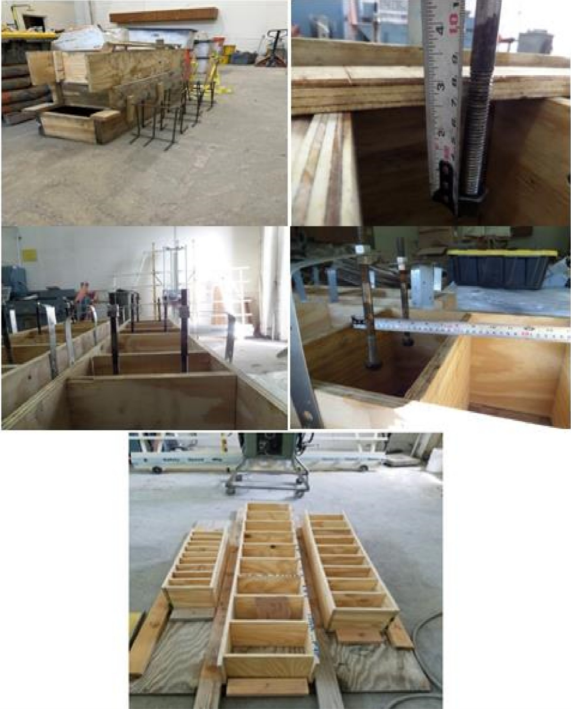
Figure 3.15 Steps of Timber Formwork Specimens
