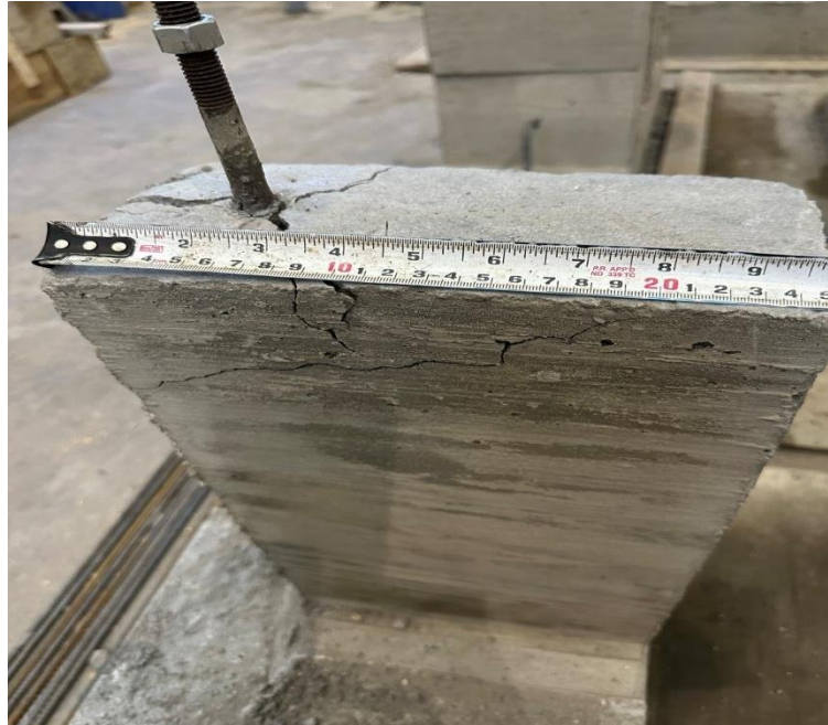
Figure 3.34 Concrete Breakout Failures (0.5% SFRC)
