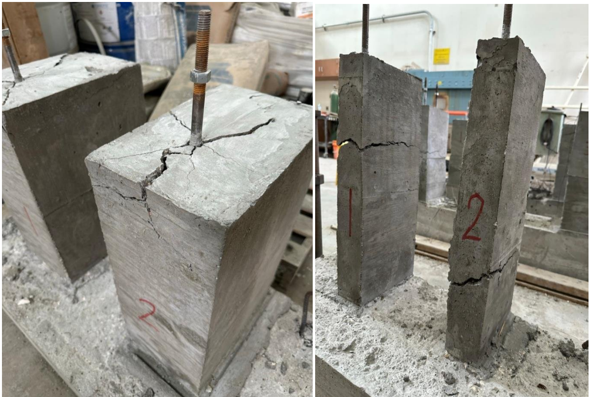
Figure 3.35 Concrete Breakout Failures (1.0% SFRC)
