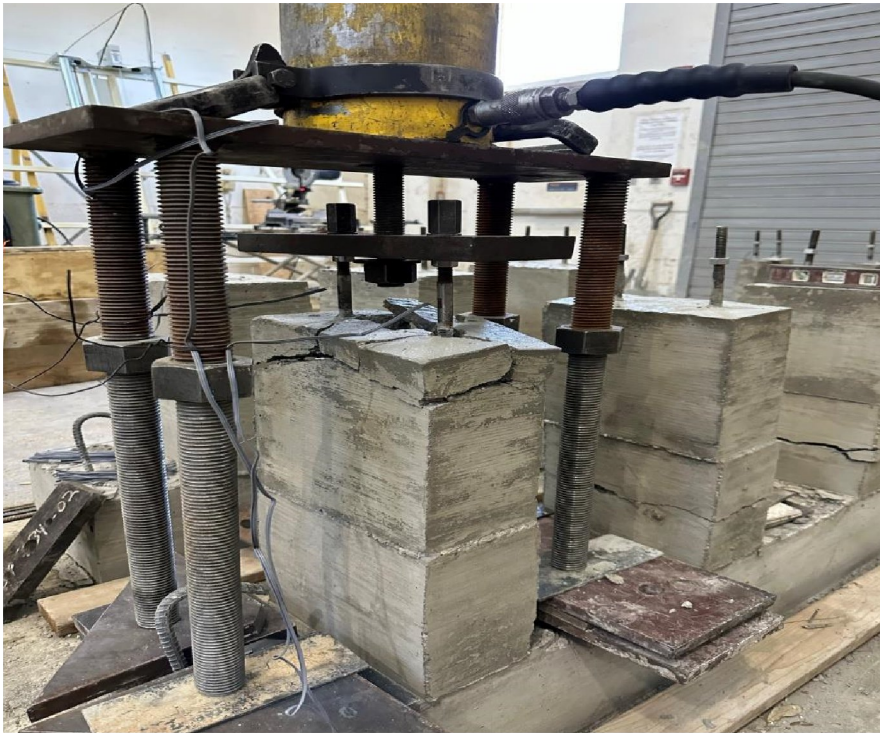
Figure 3.41 Concrete Breakout Failures (0.5% SFRC)
