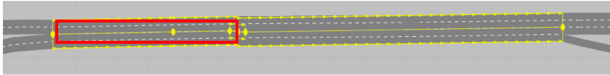
Figure 9: 500 feet High-Density Lane Change Area
