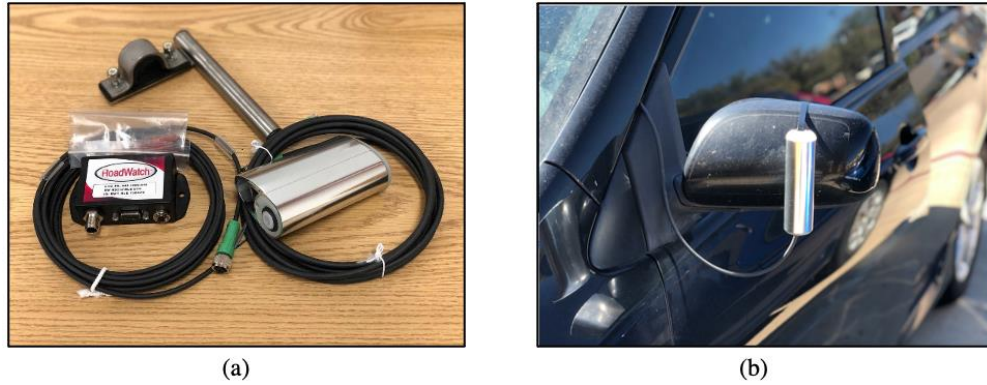
Figure 4-3 Temperature sensor used to collect road surface temperature data; (a) RoadWatch® sensor kit; (b) mounted sensor on vehicle’s side mirror
