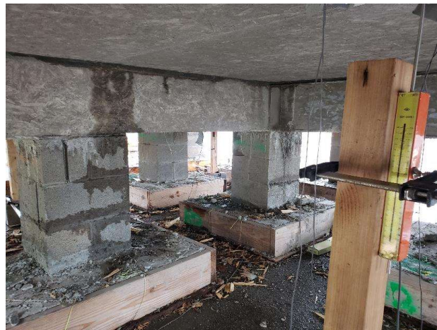
(c) Bottom Surface of Four-Panel Slab
