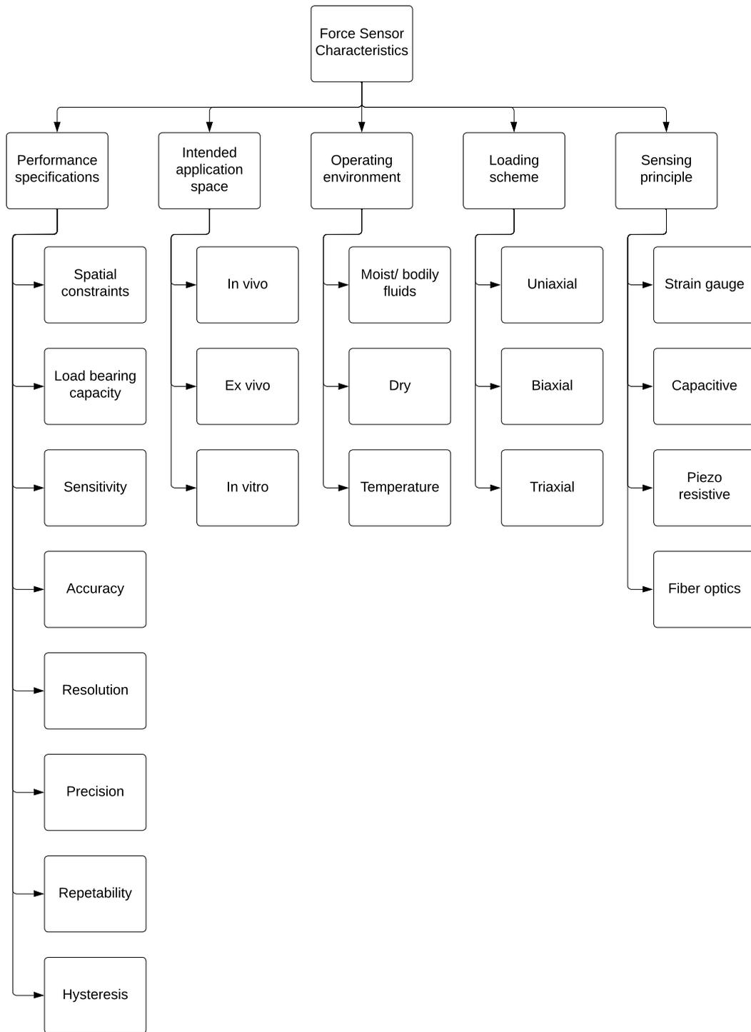
Figure 2.1: Characteristics to be considered for the development of a force sensor for medical diagnostics purposes
