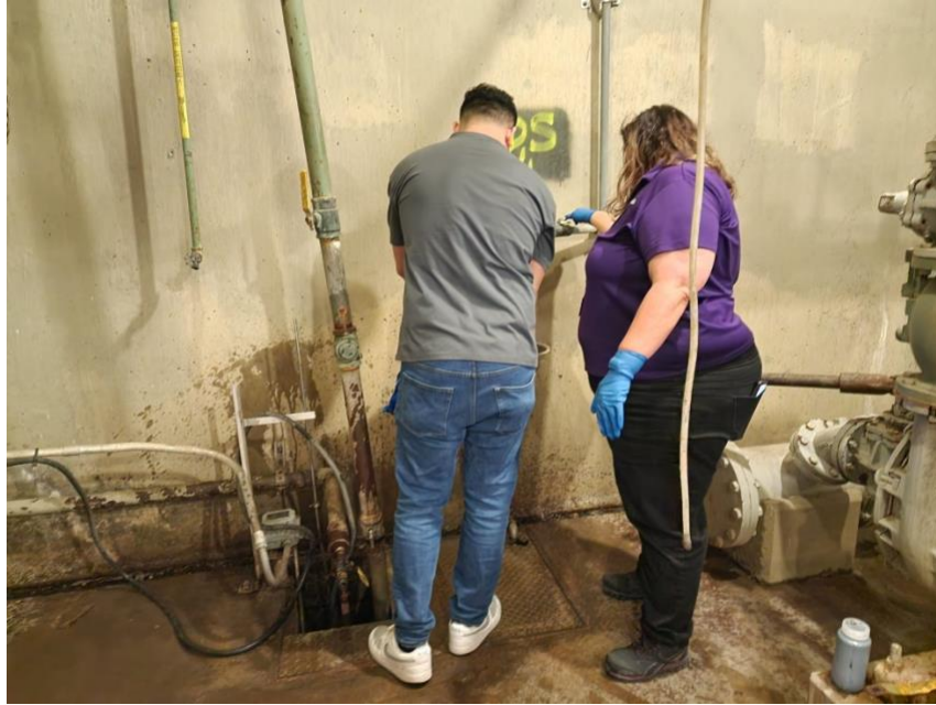
Figure 3-13: Collecting sludge from Village Creek WRRF
