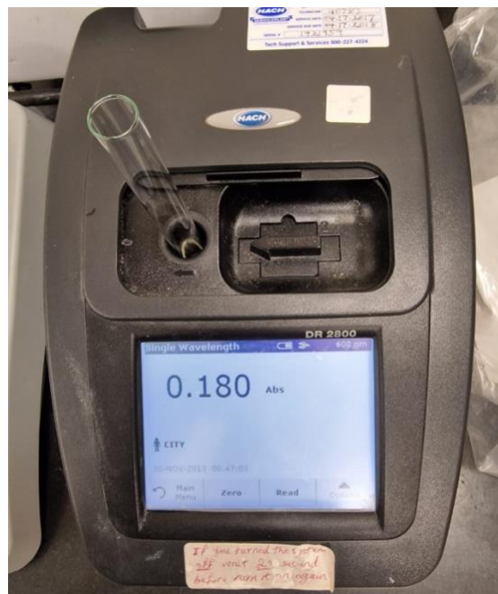
Figure 3-7: Using spectrophotometer to measure optical density of TAV5 culture
