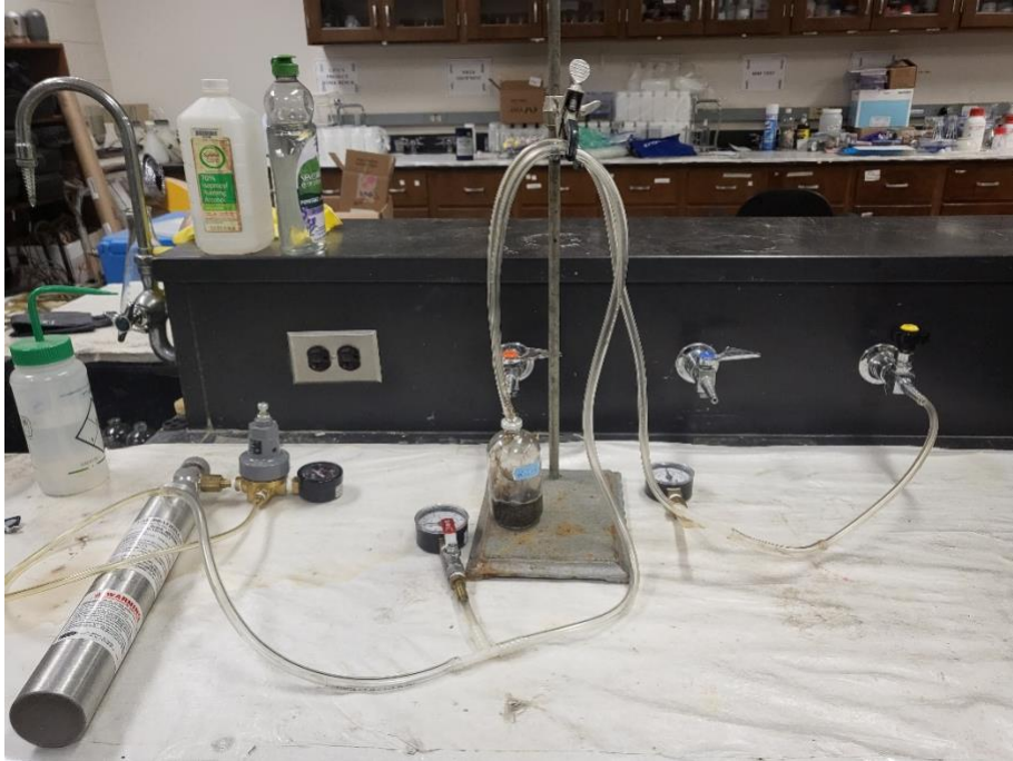
Figure 3-16: Batch reactor flushing station
