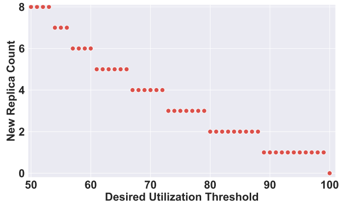
Figure 4.3: HPA calculates new instances based on desired utilization value and current utilization
