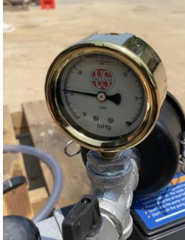
Figure 3.30 Vacuum Pressure Dial Gauge Reading (Pressure achieved 24.6-in. of Hg in Test Assembly)
