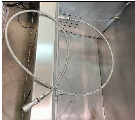
Figure 3.34 Pressure Hose in Water Bath
