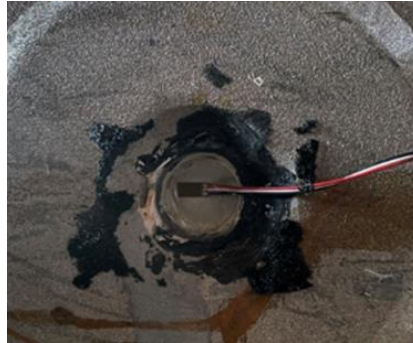
Figure 3.26 Strain Gauge Installed on 2 in. Hole Spanning
