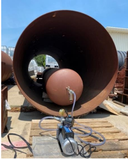
Figure 3.28 Vacuum Pressure Test Setup for 2 in. Hole Spanning Pipe Sample
