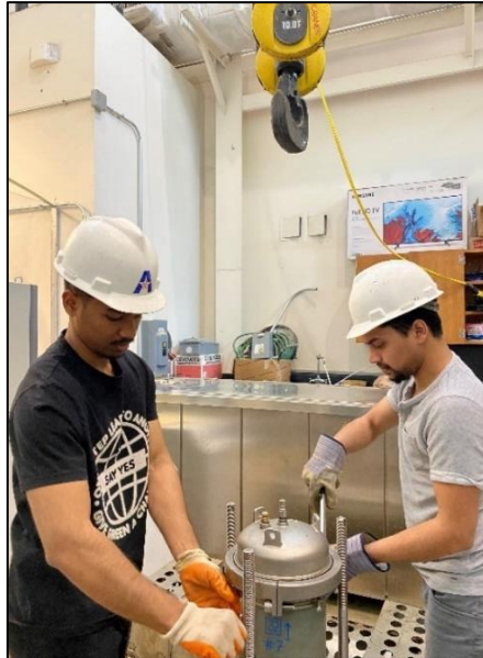
Figure 3.56 End Caps Installation in Progress
