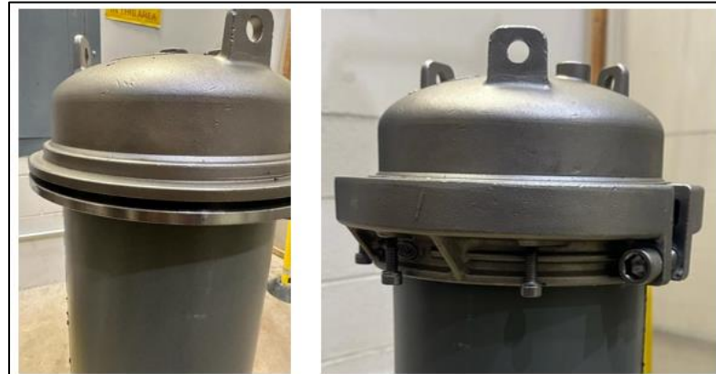
Figure 3.52 Pipe Sample with Top End Cap Installed
