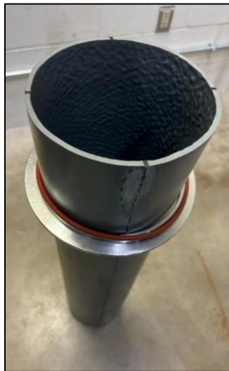
Figure 3.50 Pipe Pipe Sample with Snap Ring and O-ring
