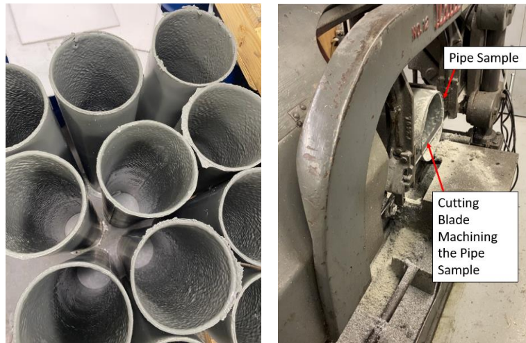
Figure 3.38 Pipe Cutting at Lathe Machine
