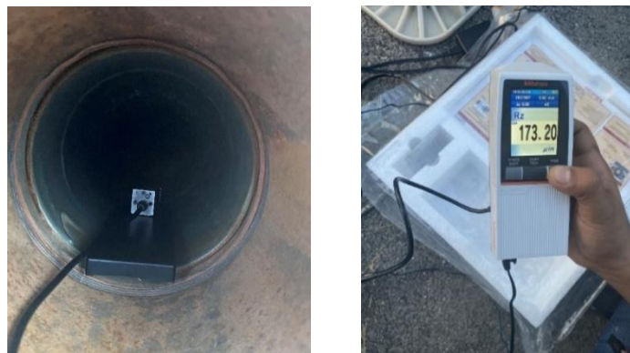
Figure 5.36 Roughness Measurement with Portable Surface Roughness Tester
