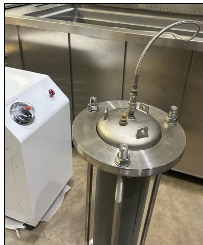
Figure 3.57 Pipe Sample Connected with Pressure Hose
