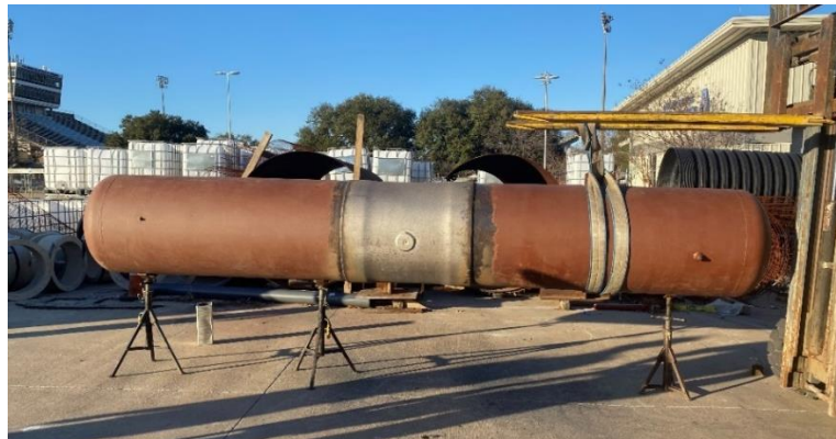
Figure 3.12 Spigot Ends Welded on Both Ends of the Test Section
