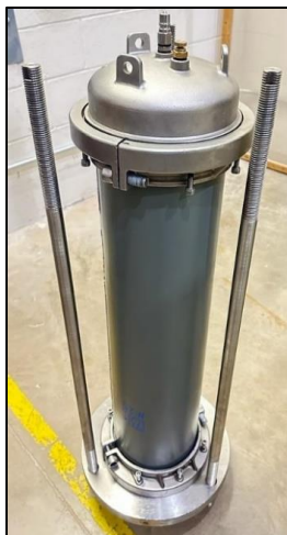
Figure 3.54 Top End Cap Installed on Pipe Sample
