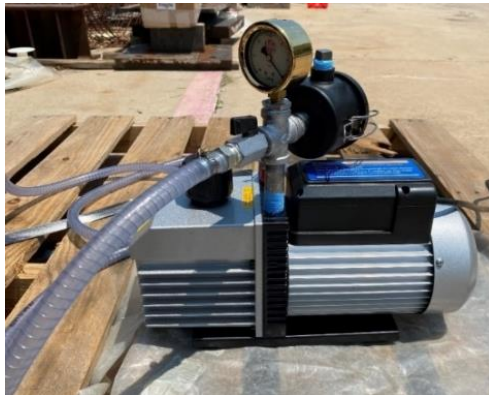
Figure 3.29 Vacuum Pressure Dial Gauge Reading (Pressure Achieved Zero in. of Hg in Test Assembly)
