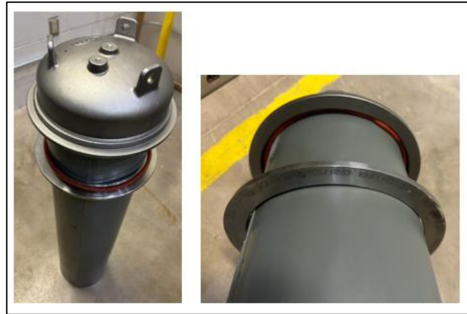
Figure 3.51 Bottom End Cap Installation in Process
