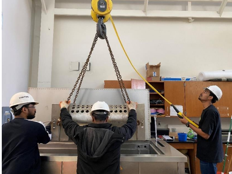
Figure 3.60 Pipe Sample Lifting with Crane
