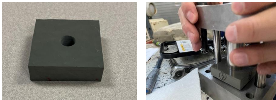
Figure 3.4 Specimen before Testing (left) Specimen Installed in Punch Shear Fixture (right)
