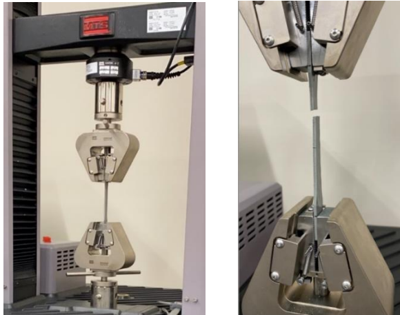
Figure 3.3 Tensile Test (left) and Specimen Rupture (Right)
