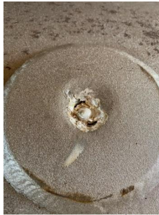
Figure 3.16 Pipe Sample with 0.5 in. Hole Spanning
