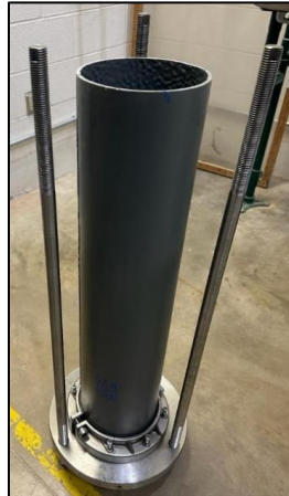
Figure 3.53 Pipe Sample with Restrained End
