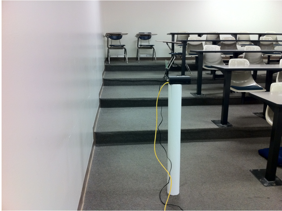
Figure 5.5. Location of the UWB radar on another side of a thick Gypsum partition wall.
