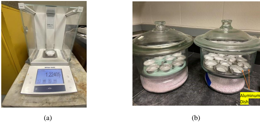
Figure 3.9: (a) Weighing balance, (b) Desiccators used for TSS measurement
