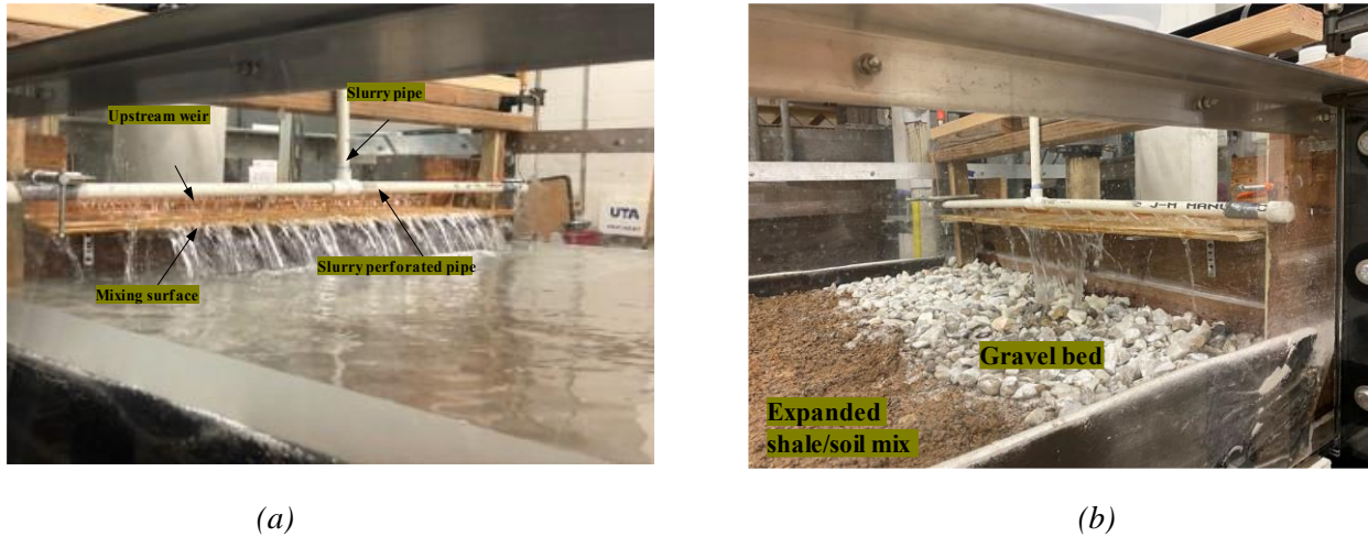
Figure 3.2: (a) Inlet section, (b) Expanded shale and upstream gravel bed
