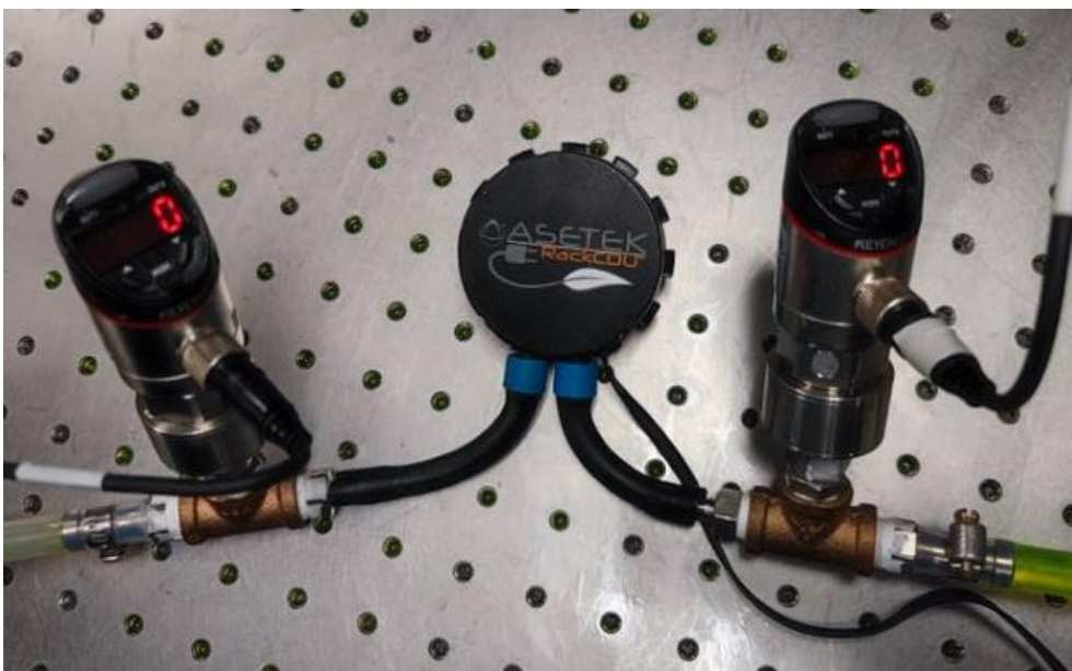
Figure 6-4 Flow resistance measurement setup
