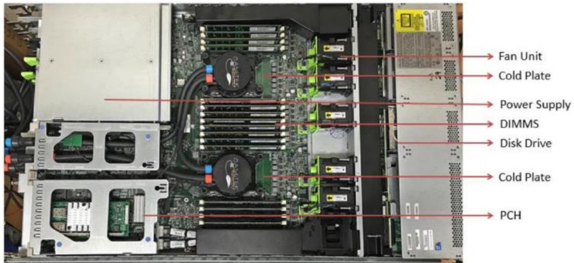
Figure 7-1 Server retrofitted with cold plates.
