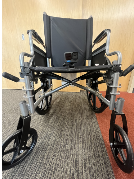
Figure 5.2: The configuration used for the experiments consists of a GoPro HERO10 camera mounted on the seat of the manual wheelchair
