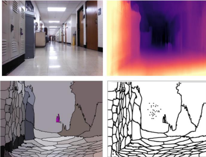
Figure 7.2: Upper row: RGB-D pair Bottom row: On the left, the DASP algorithm performs oversegmentation, dividing the image into superpixels. On the right, the seeds generated by the DASP algorithm, described by the dotted area, represent the area with the greatest depth
