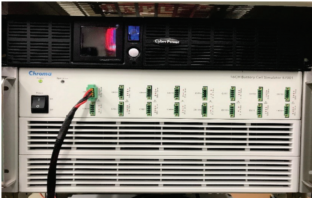
Figure 34. Chroma unit in white. It is a 16 cell emulator capable of up to 5 amps continuous current on each channel.
