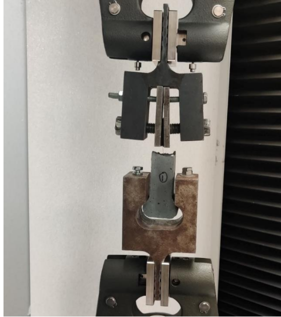
Figure 4-6 Single fiber pullout setup
