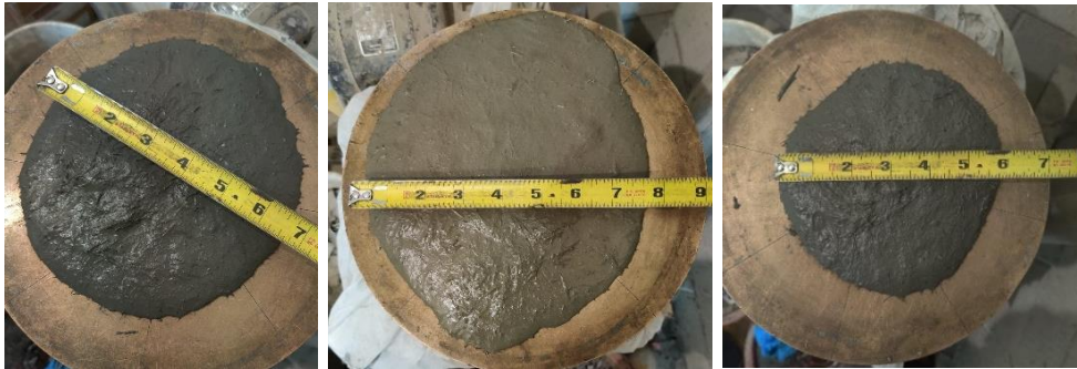
Figure 4-3 Flowability test for a. 920U, b. W940U, c. 970U
