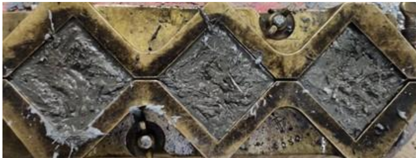
Figure 4-4 Casting of 2 in. cubes.
