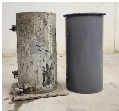
Figure 3-16 Mold for double punch test (DPT)
