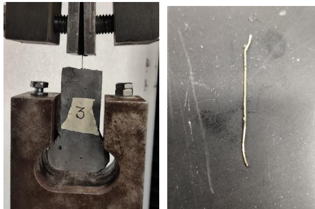
Figure 4-7 Sample test specimen for fiber pullout
