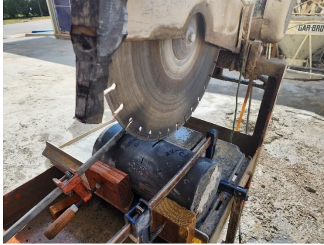
Figure 3-17 Procedure for cutting DPT cylinder specimens.
