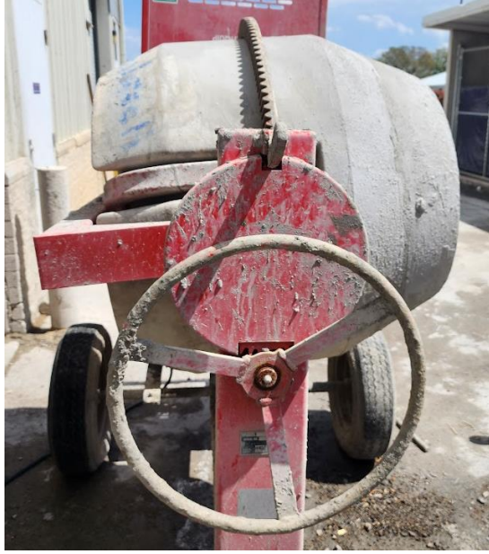
Figure 3-19 Gravity mixer for casting normal fiber-reinforced concrete.
