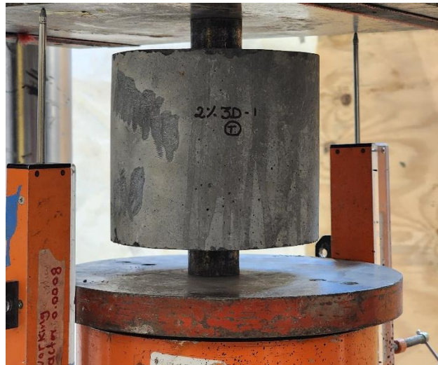
Figure 3-18 Test setup for DPT test
