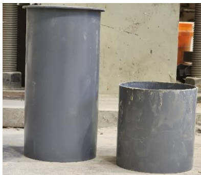
Figure 4-14 Molds cut in half.
