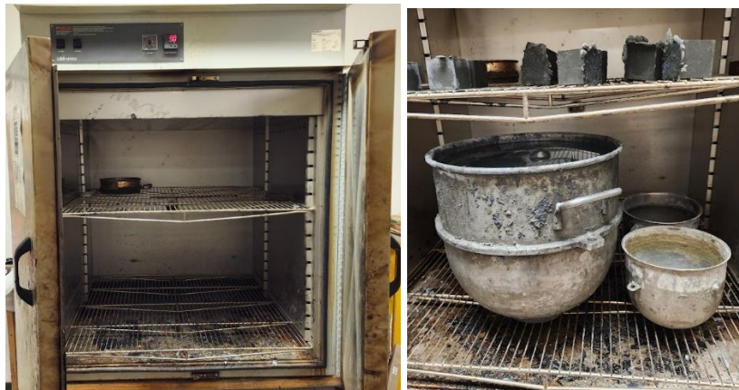
Figure 3-4 Oven used for heat treatment.
