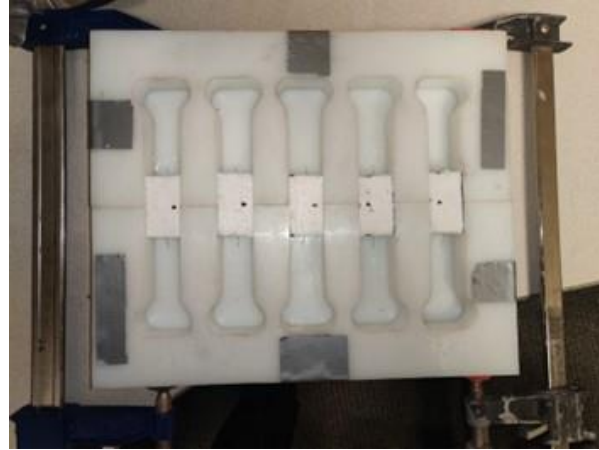
Figure 3-12 Mold for fiber pullout test
