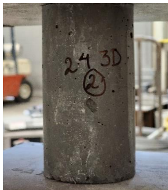
Figure 4-1 Compression test on 3×6 in. cylinders
