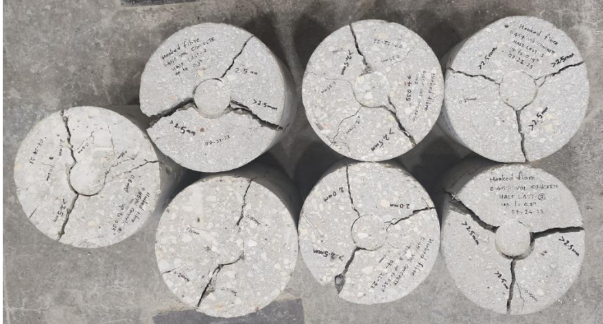
Figure 4-15 DPT specimens after failure
