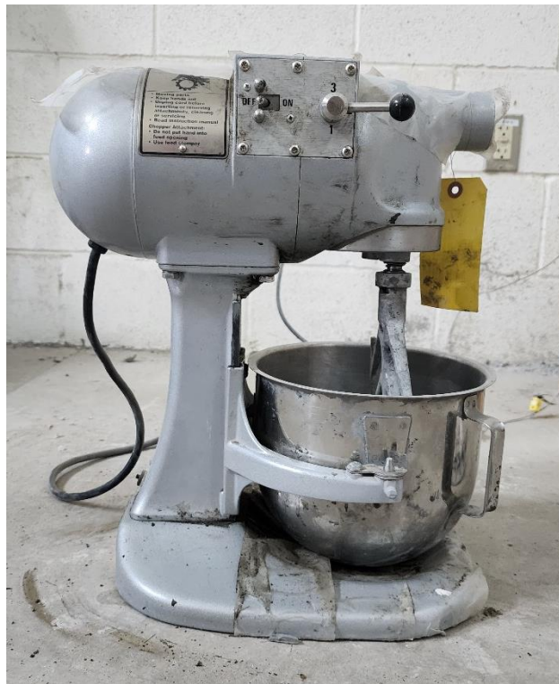
Figure 3-2 Lab mixer used for casting five quarts of UHPC.
