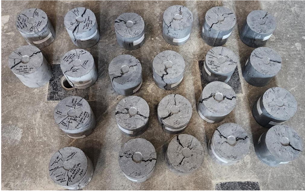
Figure 4-15 DPT specimens after testing.
