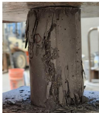
Figure 4-1 Compression test on 3×6 in. cylinders
