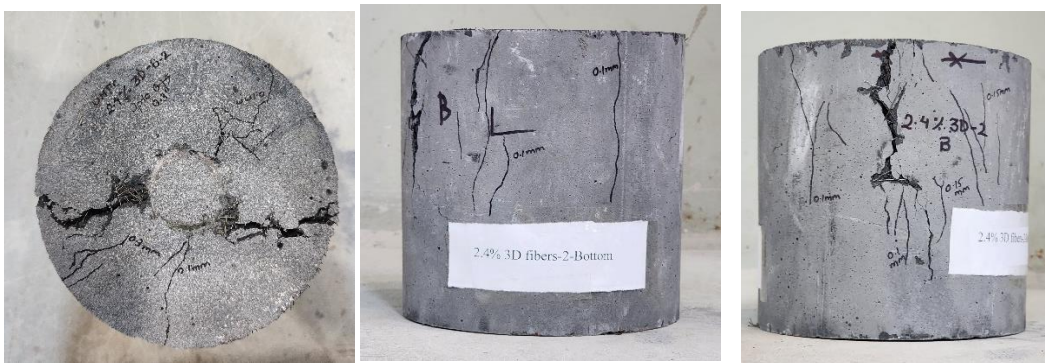
Figure 4-14 Sample DPT specimen showing cracks.
