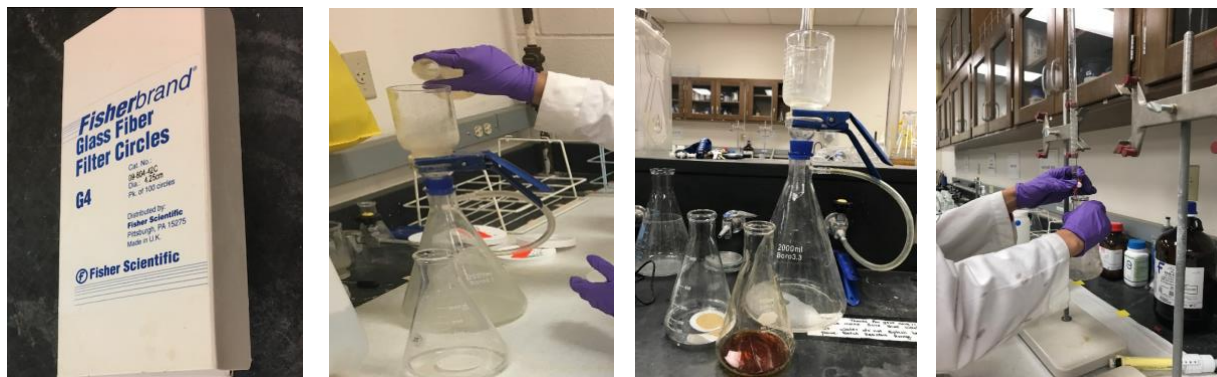
Fig 3.10 Vacuum filtration of the sample and iodometric method for sulfide determination
