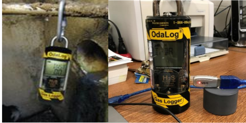
Fig 3.3 OdaLog SL 50 (App-Tek International) in the manhole and OdaLog with the IrDA
