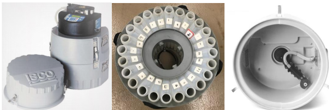
Fig 3.8 ISCO 6712 Full-Size Portable Sampler with 24 bottles of 500 ml volume and Adjustable Distributer Arm
