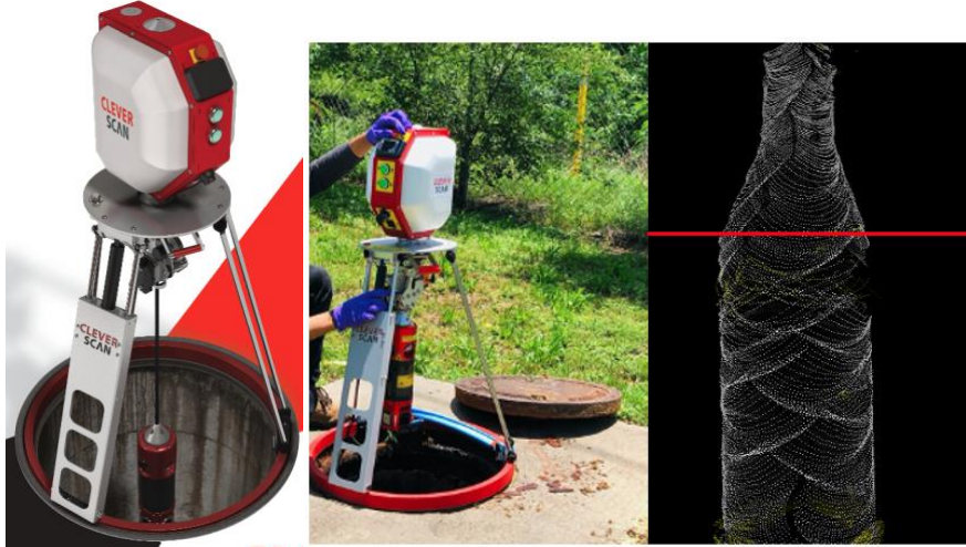
Fig 3.15 CleverScan being used in the field for manhole diameter measurement and the point cloud
