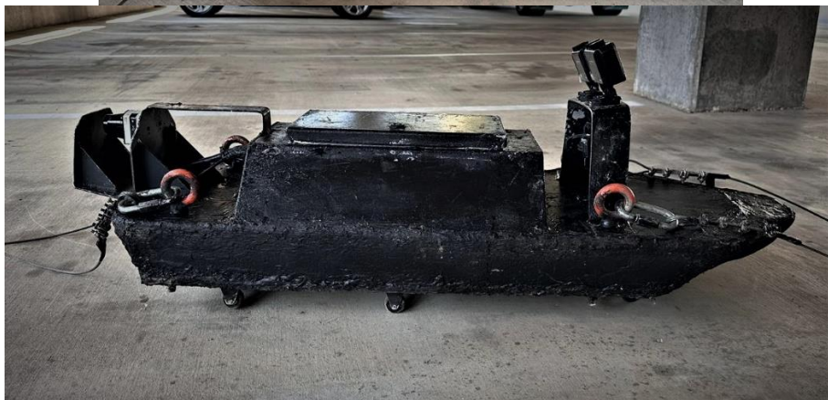
Figure 3-7 Multi Sensor robotic boat (MSI) third version for large size pipes designed and built by CSER/MSI
