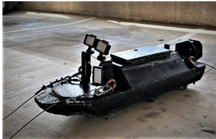
Figure 3-6 Multi Sensor robotic boat (MSI) second version for larger size pipes designed and built by CSER/MSI
