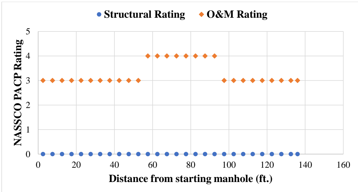
Figure 4-27 NASSCO's PACP rating for every five feet pipe segments in Line_11080
