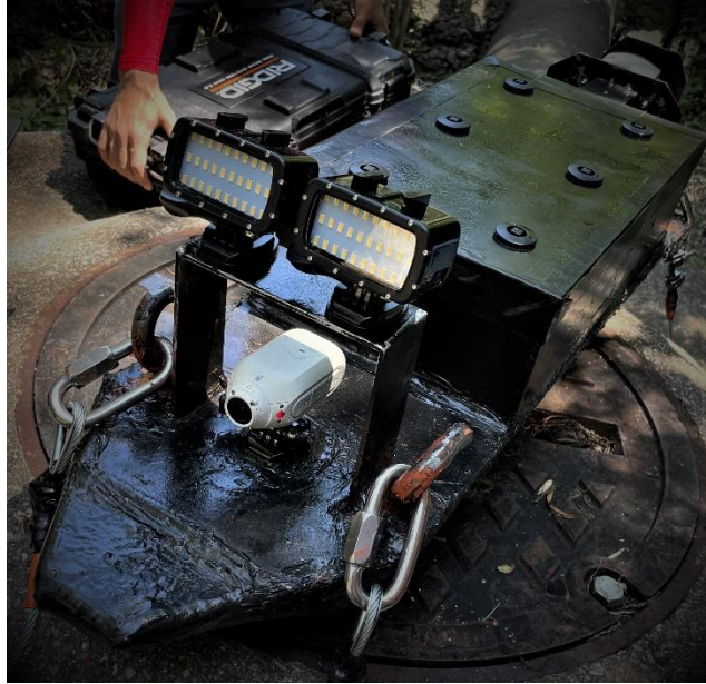
Figure 3-8 Multi Sensor robotic boat (MSI) third version for smaller size pipes designed and built by CSER/MSI
