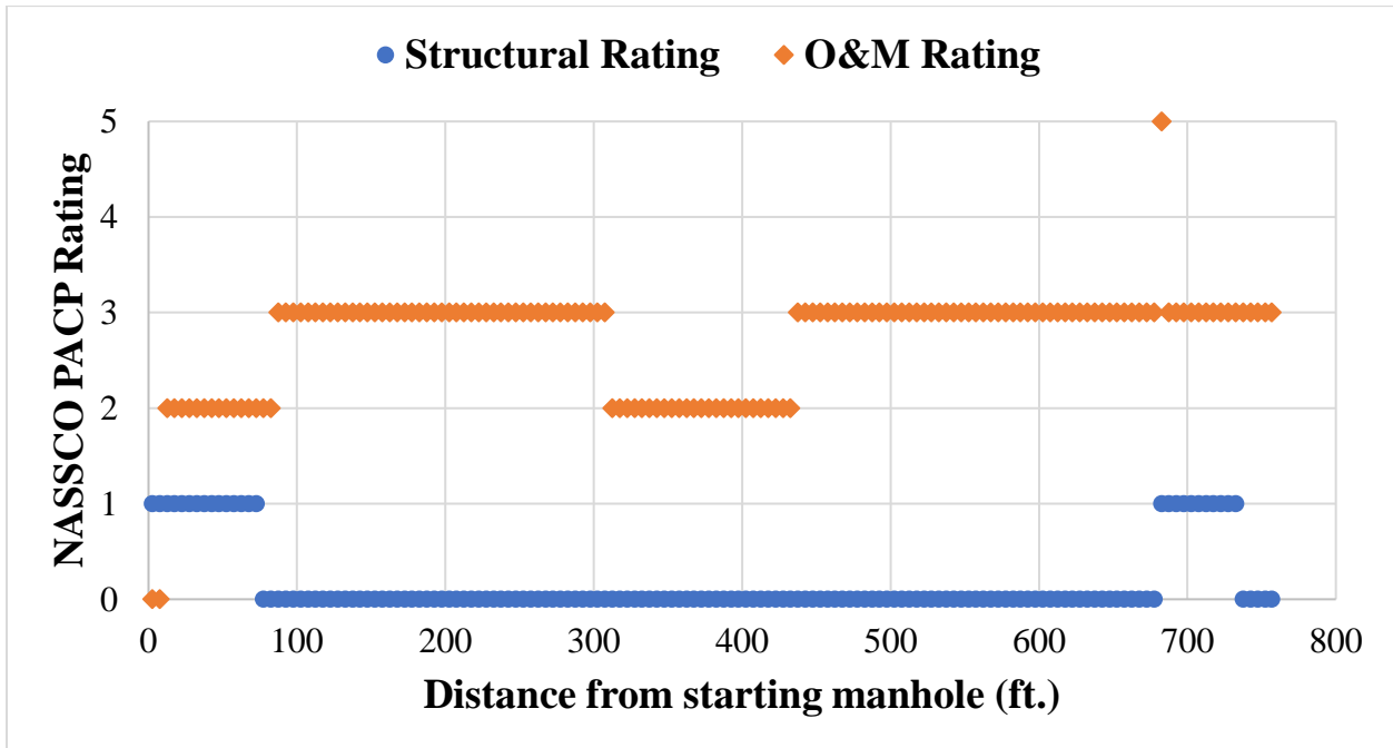
Figure 4-33 NASSCO's PACP rating for every five feet pipe segments in Line_11084
