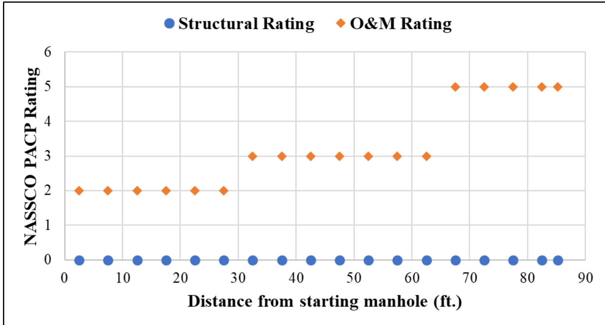
Figure 4-24 NASSCO's PACP rating for every five feet pipe segments in Line_12890
