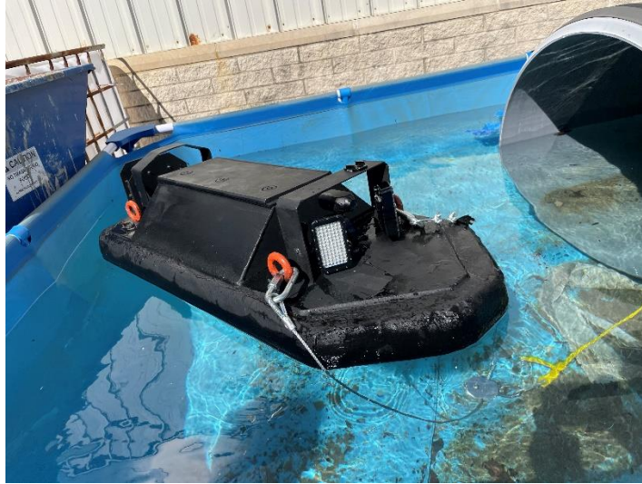
Figure 3-6 Multi Sensor robotic boat (MSI) second version for larger size pipes designed and built by CSER/MSI
