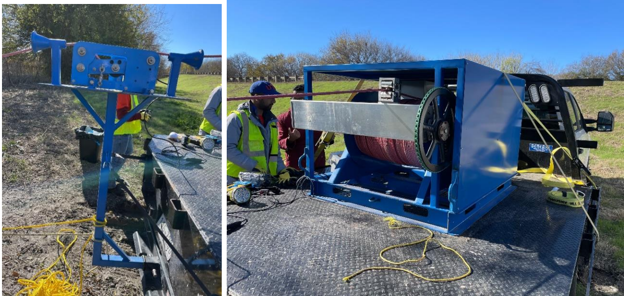
Figure 3-3 The Counter and Counter stand mounted on truck bed.
