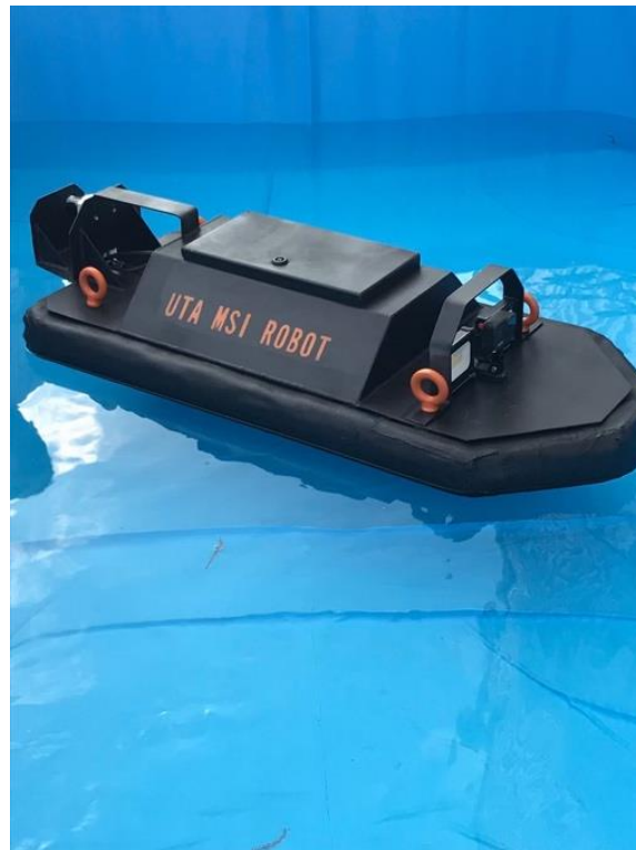
Figure 3-5 Multi Sensor robotic boat (MSI) designed and built by CSER/MSI
