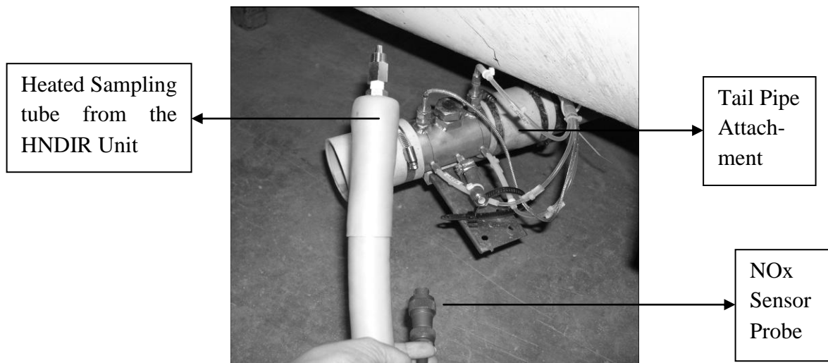
Figure 3.7 Sampling and NO x sensor tube attached to the tail pipe attachment
