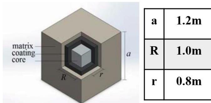
**Figure 2-1:** 3D-3C unit cell (Shi and Huang, 2013).
