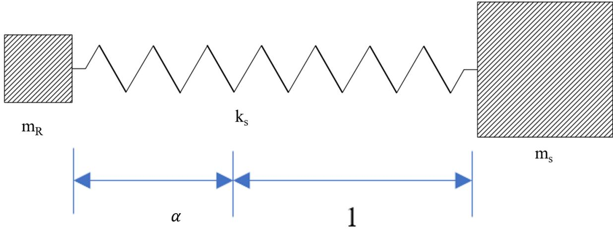
**Figure 4-24:** Spring-mass-spring equivalent model.
