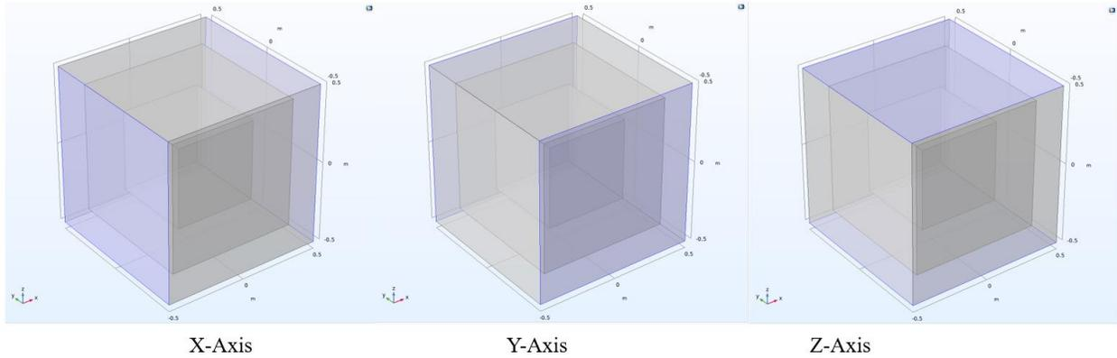
**Figure 4-1:** Assigned PBC for a 3D-3C unit cell.
