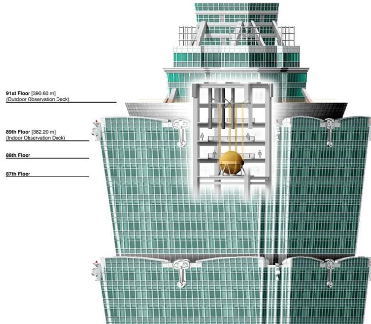
**Figure 1-10:** Taipei 101 building TMD (<https://www.slate.com>, accessed 2023).
