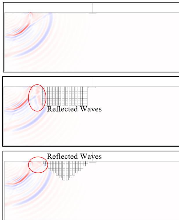
**Figure 4-58:** Wave contours generated by Ormsby wavelet at 0.7 seconds with different configurations (Top) soil medium without protection, (Mid) protection using a double-graded array, and (Bottom) protection using a double-graded pyramid.
