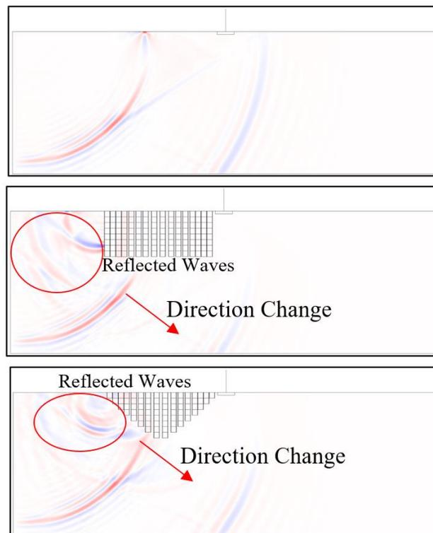
**Figure 4-59:** Wave contours generated by Ormsby wavelet at 1.1 seconds with different configurations (Top) soil medium without protection, (Mid) protection using a double-graded array, and (Bottom) protection using a double-graded pyramid.
