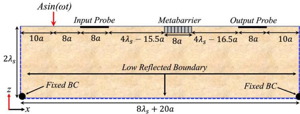
**Figure 3-21:** Time transient analysis FEA (Muhammad et al., 2021).
