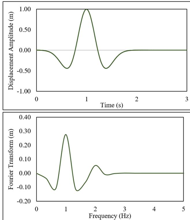
**Figure 3-19:** Ricker wavelet and its Fourier transform function.
