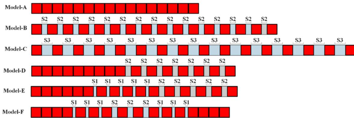
**Figure 3-25:** Proposed unit cell configurations for bandgap manipulation.
