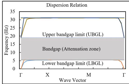
**Figure 1-18:** Typical dispersion relation for metamaterial unit cell.
