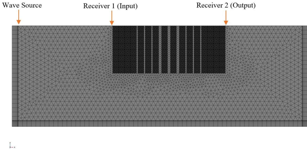
**Figure 3-16:** Mesh of the full-scale dynamic response analyses.
