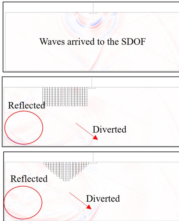
**Figure 4-60:** Wave contours generated by Ormsby wavelet at 1.7 seconds with different configurations (Top) soil medium without protection, (Mid) protection using a double-graded array, and (Bottom) protection using a double-graded pyramid.
