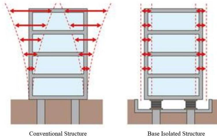
**Figure 1-9:** Base isolation system implementation (Verma et al., 2017).
