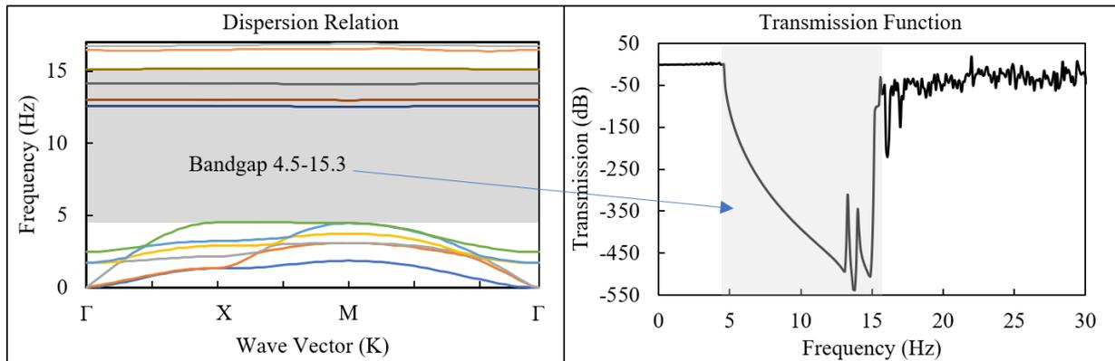
**Figure 4-26:** Dispersion relation and Transmission of type II unit cell.
