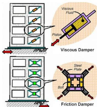
**Figure 1-8:** Viscous damper example (mathspig.wordpress.com, accessed 2023).
