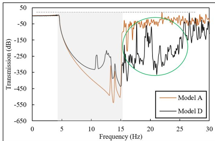
**Figure 4-30:** Comparison of Transmission between model-A and model-D.
