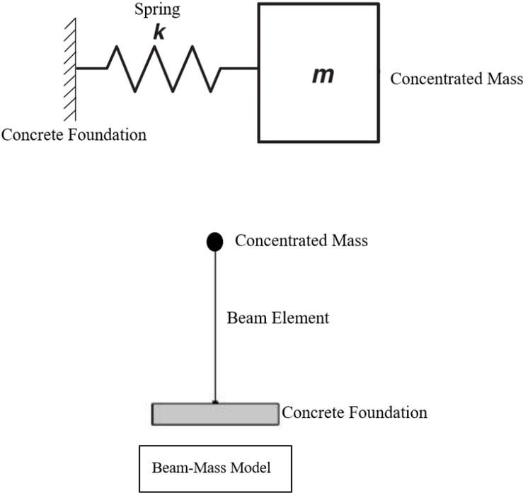
**Figure 4-40:** Methods of modeling the SDOF structure.
