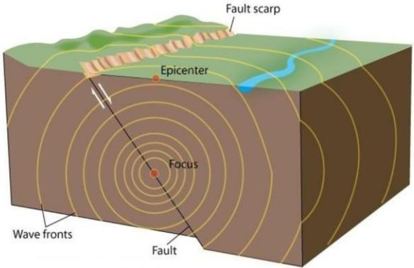
**Figure 1-1:** Earthquake waves (University of Waikato, accessed 2023).
