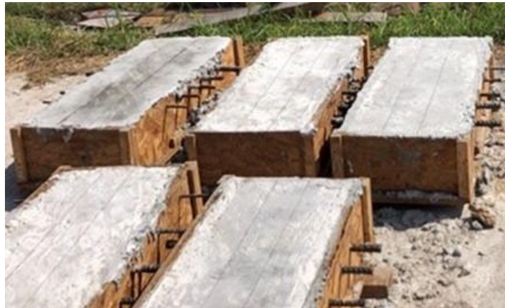
Figure 3- 4. Concrete specimens with rebar embedded
