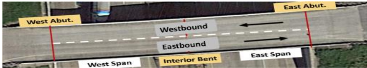
Figure 4- 17. I-45 Bridge plan view
