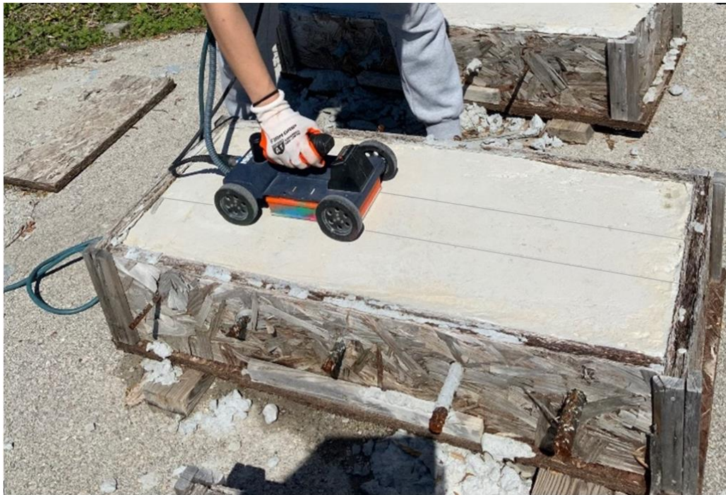
Figure 2- 8. RC specimen scanning
