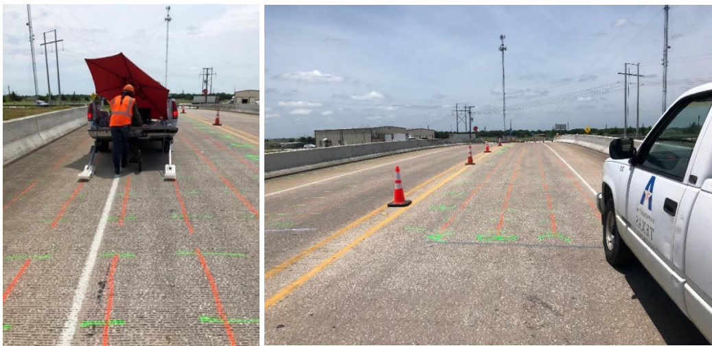
Figure 4- 18. GPR scanning path over the I-45 Bridge deck
