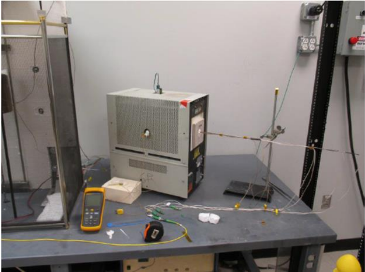
Figure 2.5. Furnace And Experimental Setup for Determining High Temperature Coefficients.
