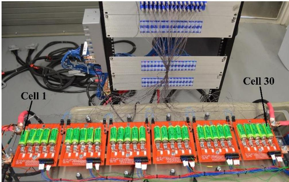
Figure 5: 1S/30P battery and thermocouple input ports
