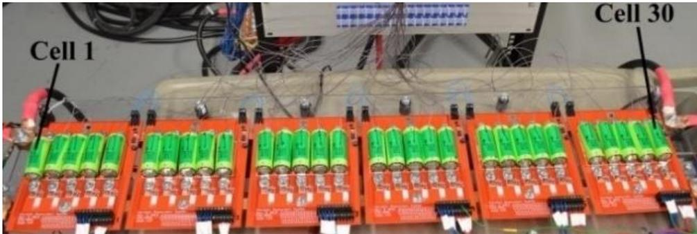
Figure 9: 1S/30P battery and thermocouple input ports
