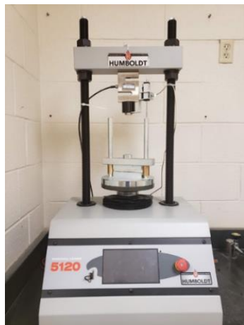
Figure 3.12 Test Set-Up for Indirect Tensile Strength Test
