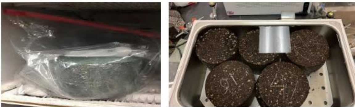
Figure 3.13 Conditioning (freezing thawing) the samples to determine TSR for moisture susceptibility test
