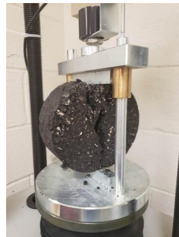
Figure 3.12 Test Set-Up for Indirect Tensile Strength Test
