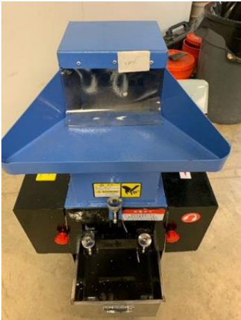
(b) Laboratory shredding machine to shred HDPE and PP
