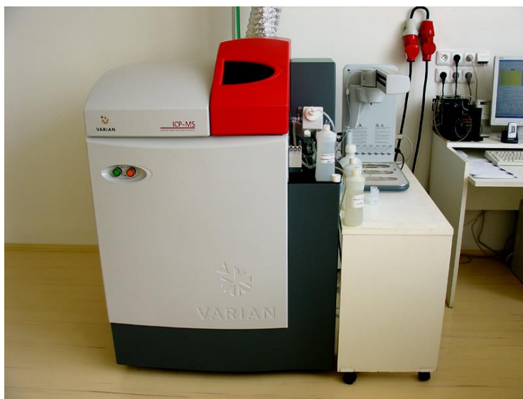
Figure 2.17 Analytical instrument ICP-MS from Varian company
