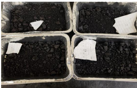
Figure 3.8 Loose (left) and compacted (right) samples for the tests
