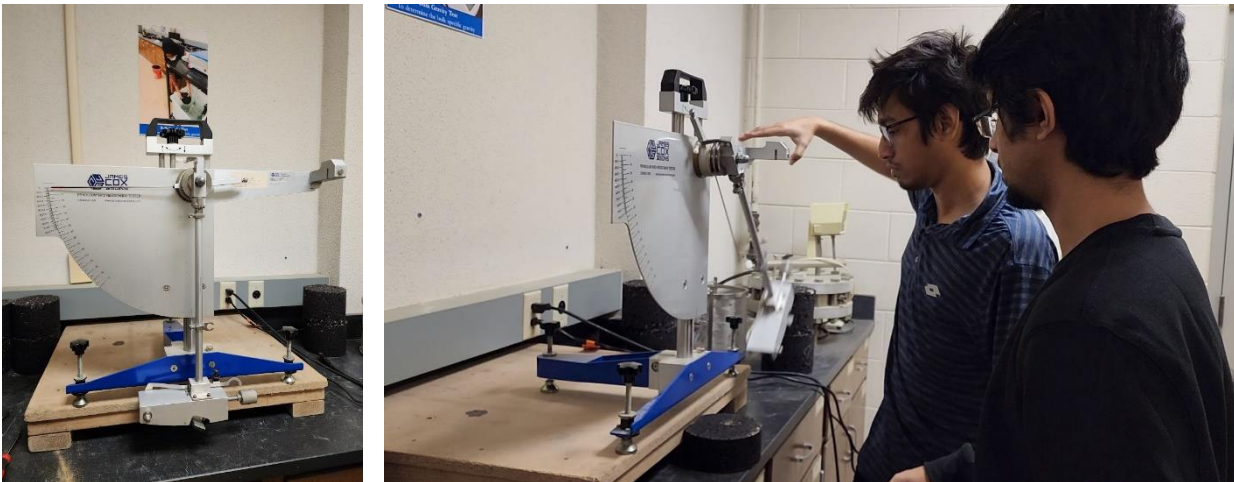
Figure 3.14 Skid resistance test setup and the procedure
