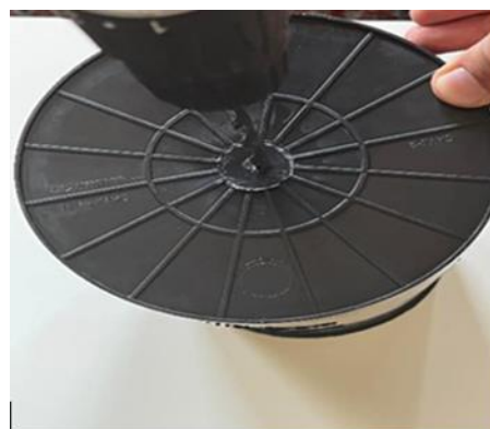
Figure 37. Making a Hole at the Bottom of the Cylinders
