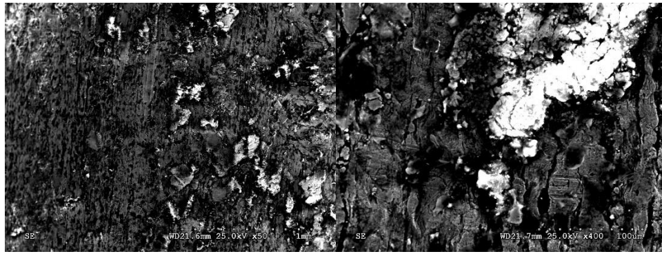
Figure 55. SEM for 0.01" Crack Width at the Control and 100,000 ppm Under (a) 50x and (b) 400x Magnification
