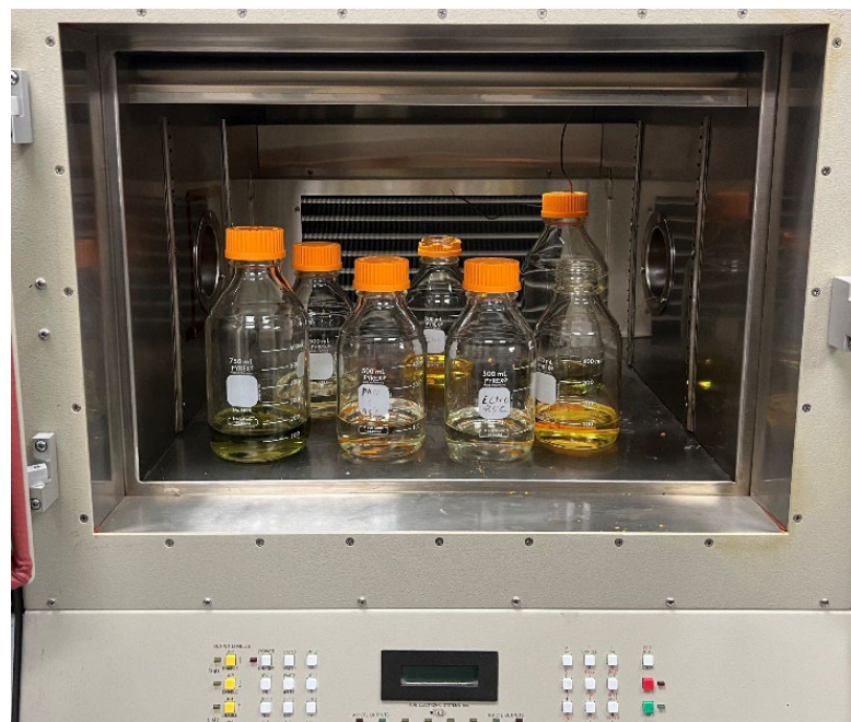
Figure 4.3: Sample bottles placed in a thermal chamber
