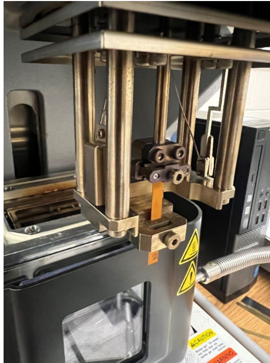
Figure 4.2: Sample mounted in the tensile attachment on DMA
