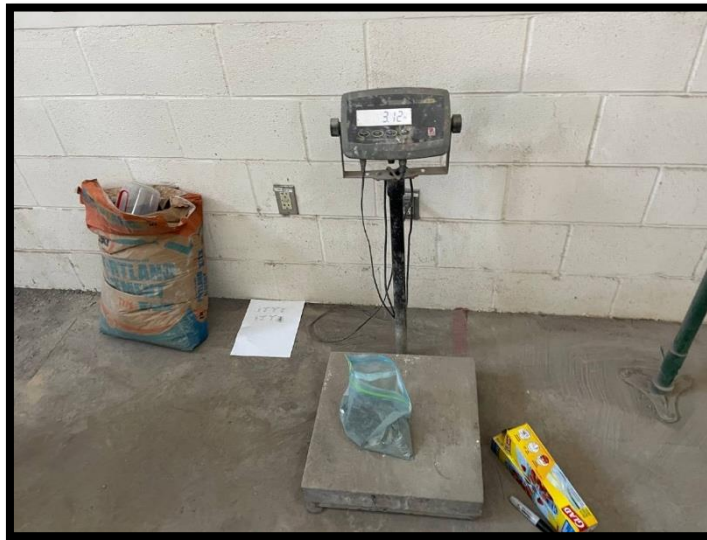
Figure 3-6 Measuring Type I/II Cement Used in the Experiments
