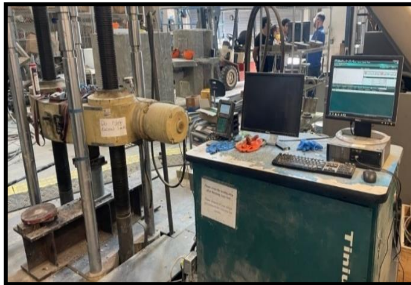
Figure 3-11. Compressive Strength Testing
