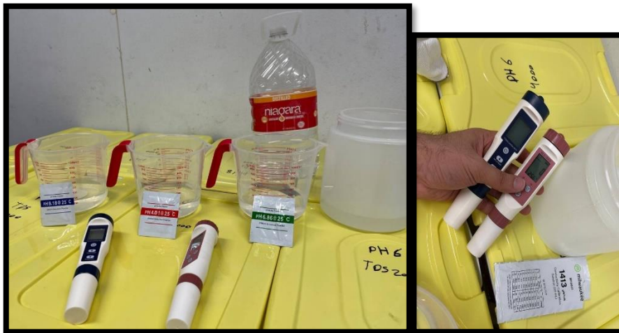
Figure 3-7 Water Testers, pH Meter, and TDS Meter
