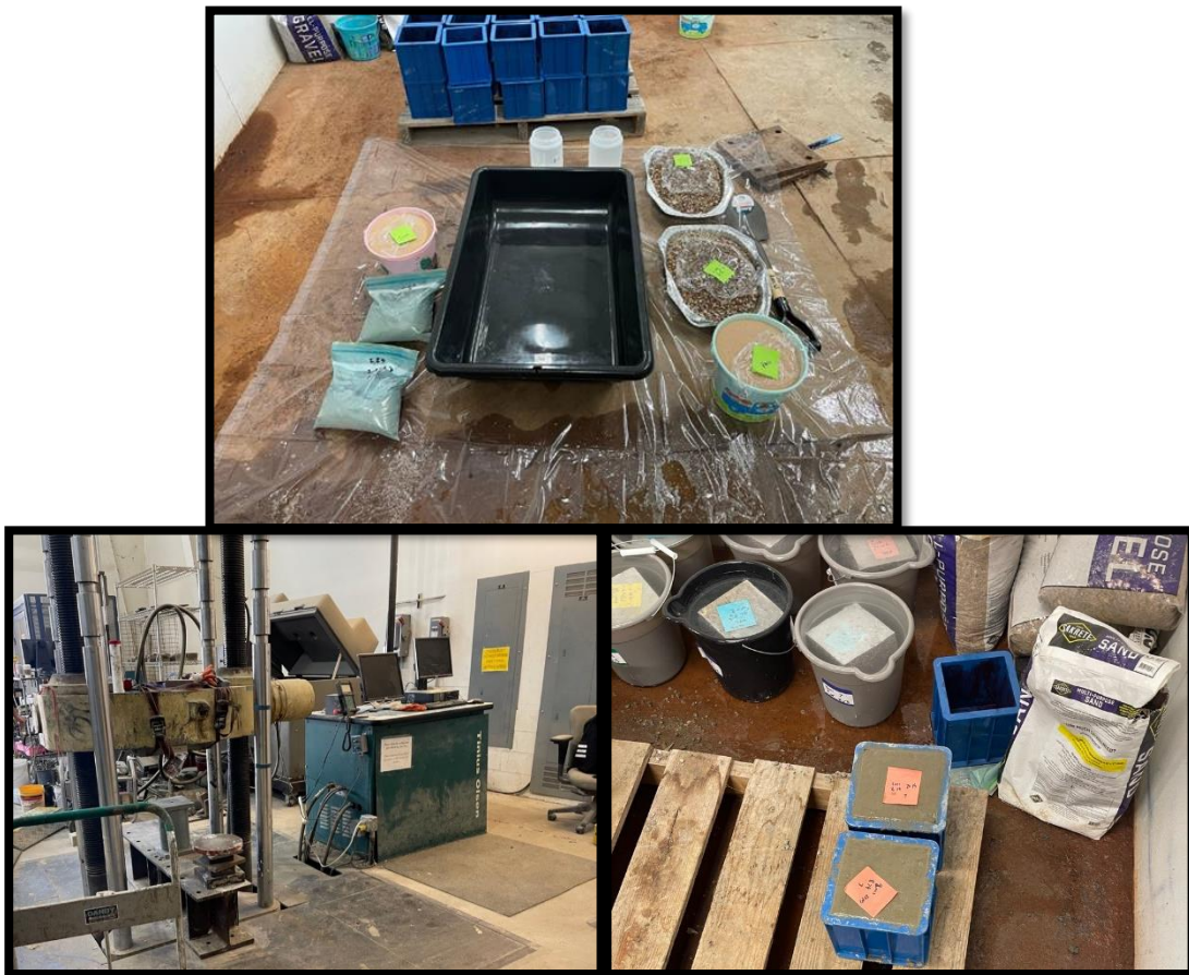
Figure 3-9 Preparation and Mixing of Concrete Used in Sample 0.6
