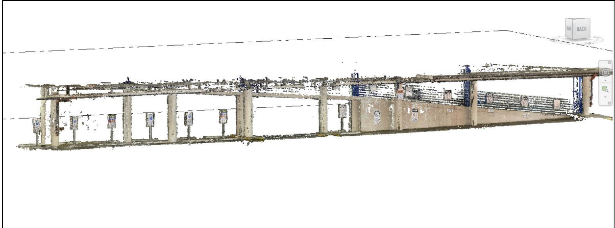
Figure 5.27. RCP point cloud in Revit
