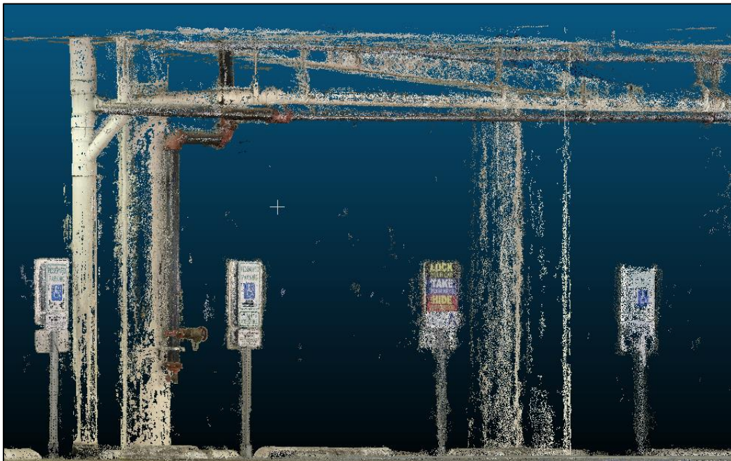
Figure 2.9. RGB point cloud reconstructed from iPhone images
