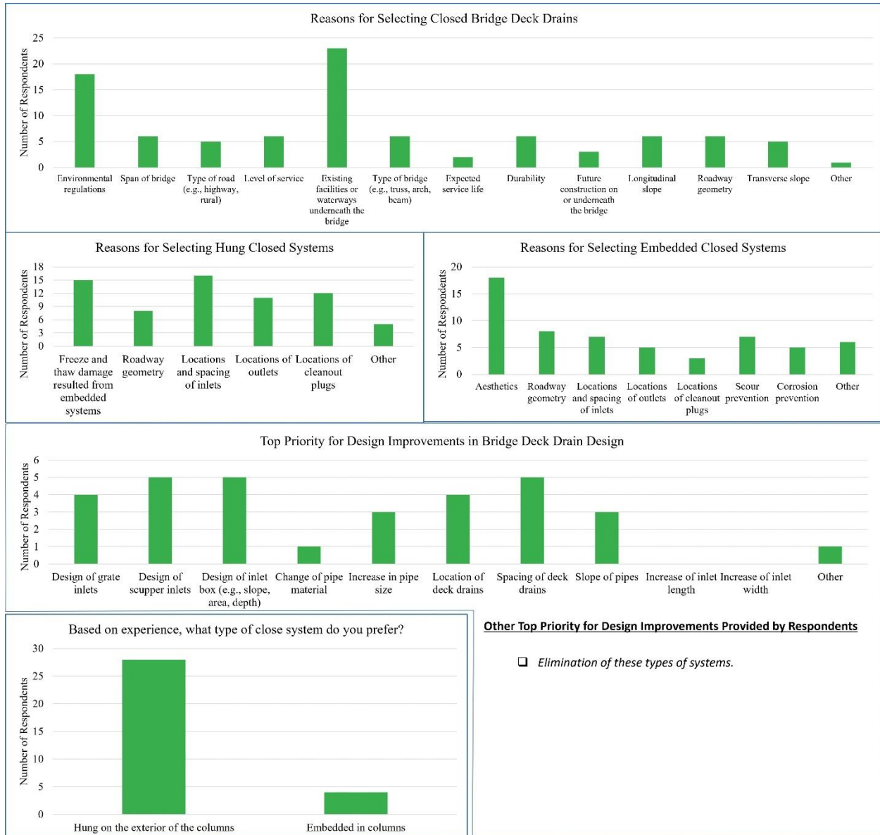
Figure 11.6. Summary of survey responses on bridge deck drain design (outside Texas)
