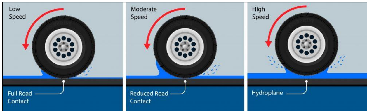
Figure 2.5. Tire hydroplaning at different speeds and water depth (left) No hydroplaning occurs (middle) Tires start losing contact with road (right) Tire no longer has contact with road (Smartmotorist, 2022)
