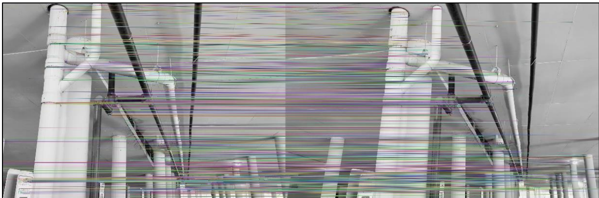
Figure 2.14. Feature matching between 2D images using SIFT descriptors
