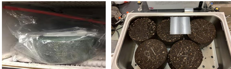
Figure 3.21. Conditioning (freezing thawing) the samples to determine TSR
