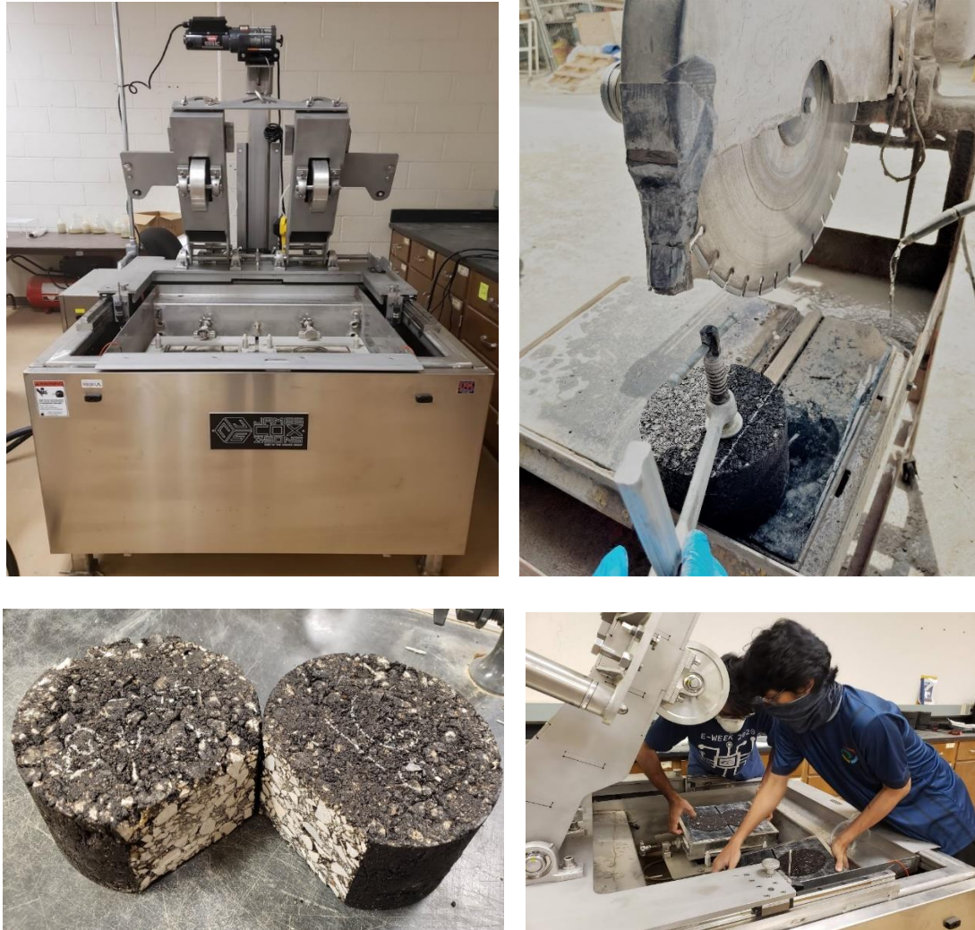
Figure 3.16. Hamburg Wheel Tracking Test
