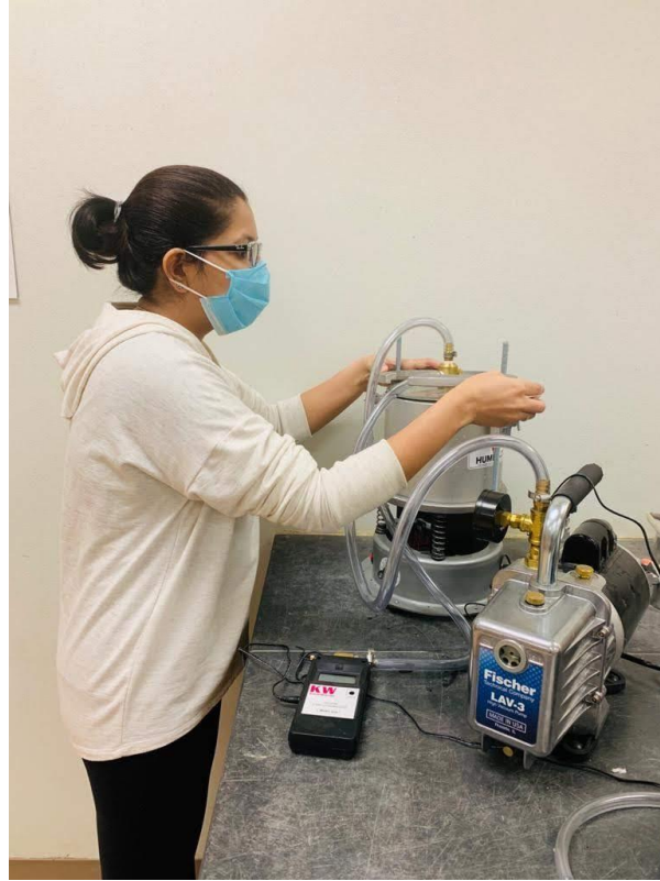
Figure 3.15. Determination of Theoretical Maximum Specific Gravity
