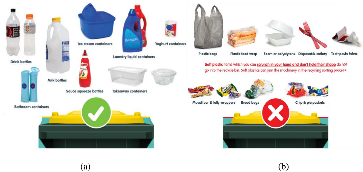
Figure 2.16. (a) Recyclable plastics (Grade #1, #2 and #5) (b) Non-recyclable plastics (Grade #4, #6 and #7) (Whitehorse Recycling Book, 2020)
