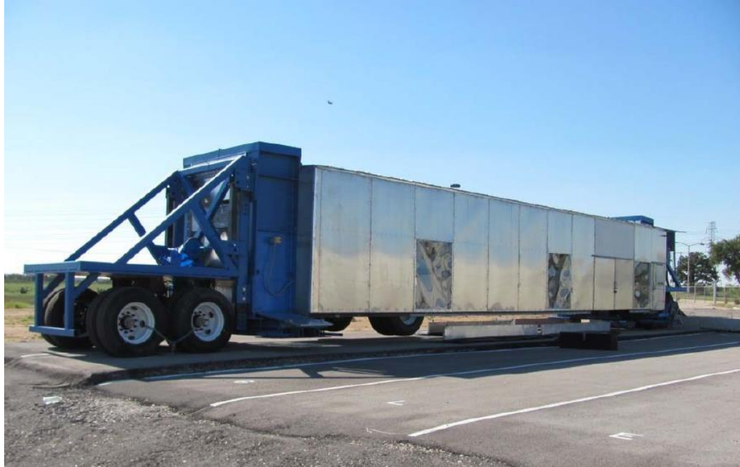
Figure 3.2 Pavement Testing Machine
