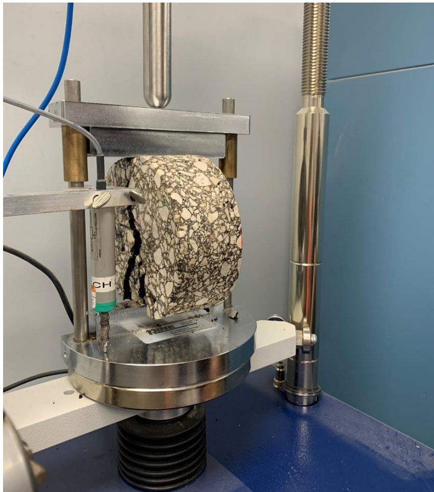
Figure 4.33 Testing setup for the IDEAL-CT Test
