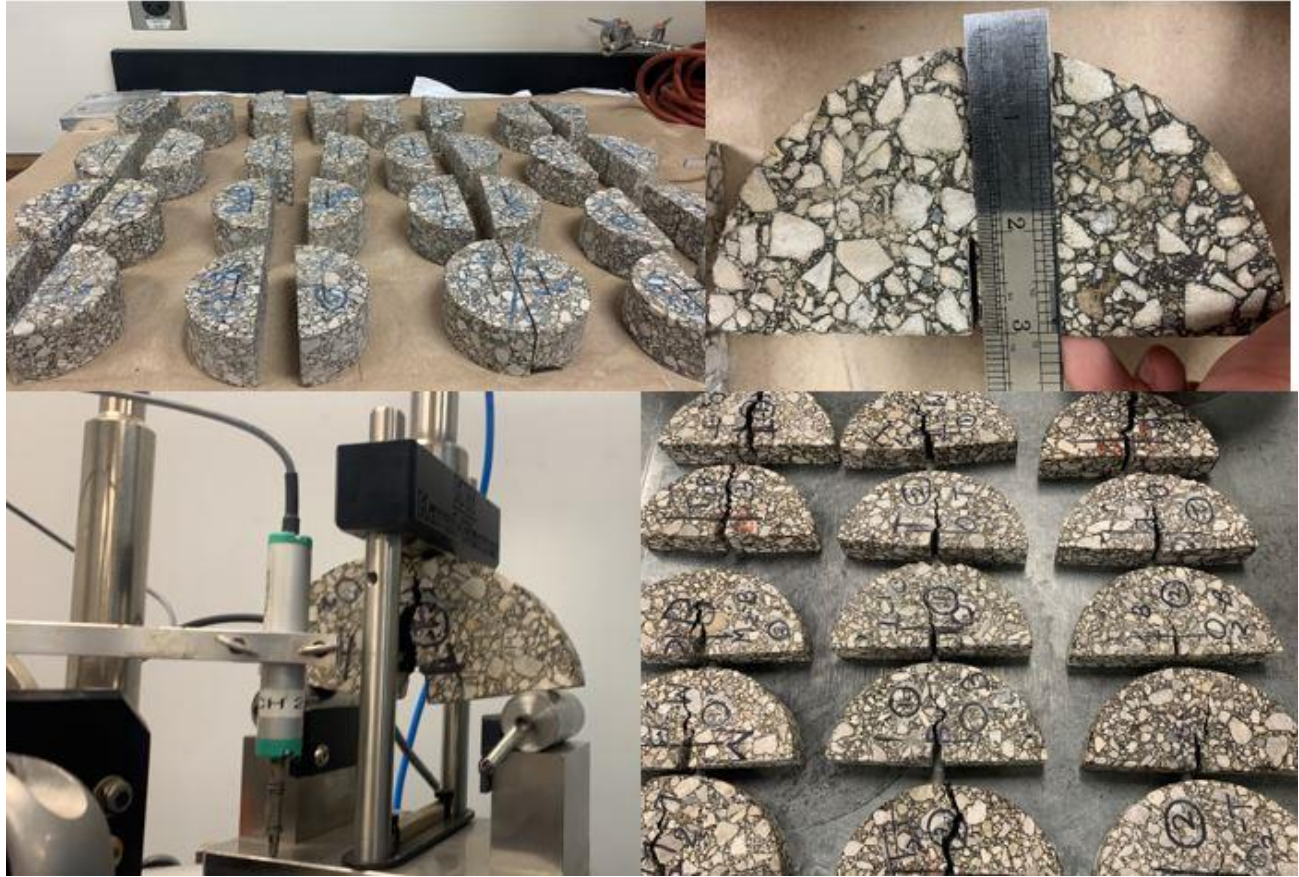
Figure 4.37 SCB Test setup and failed specimens
