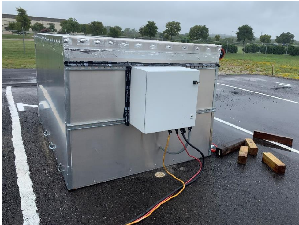
Figure 3.37 Small artificial aging box
