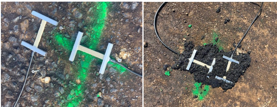
Figure 3.20 Strain gauges on Sections M
