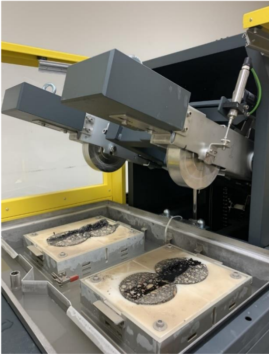
Figure 2.8 Hamburg Wheel Tracking Test
