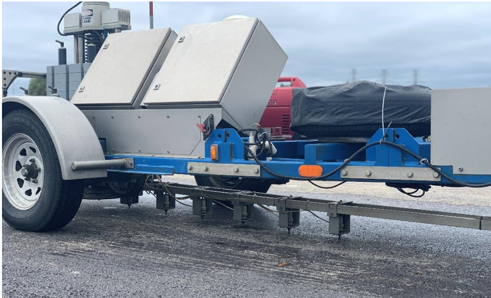
Figure 3.35 FWD testing on Section M
