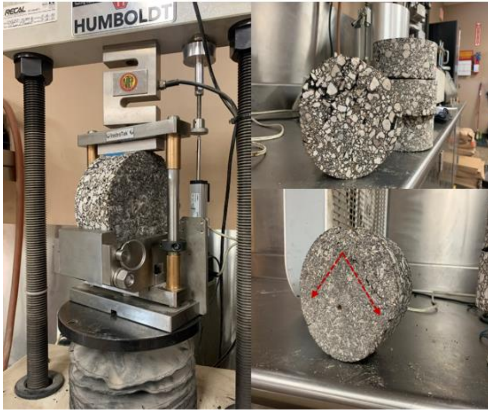
Figure 4.16 IDEAL-RT Test setup and failed specimens
