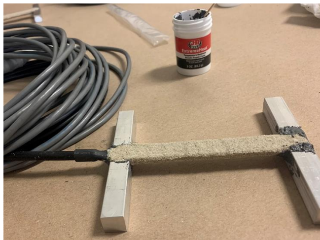
Figure 3.18 Strain gauge, model PMFLS-60-50-2LTSC, Tokyo Sokki
