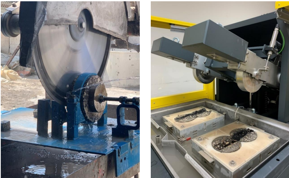
Figure 4.5 Cutting of the specimens and testing assembling in the HWT device
