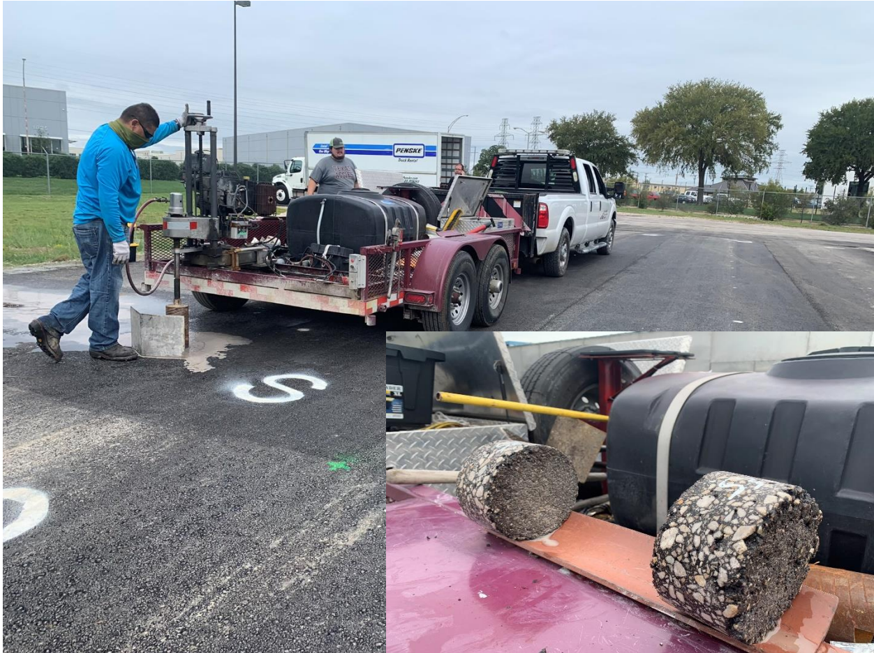
Figure 3.29 TTI extracting cores from Section S
