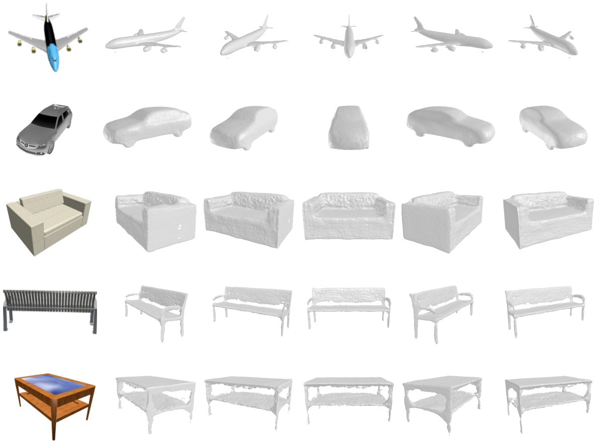
Figure 5.1: Five unique views of objects reconstructed by LIST from a single RGB image. Not only does our model accurately recover occluded geometry, but also the reconstructed surfaces are not influenced by the input-view direction.
