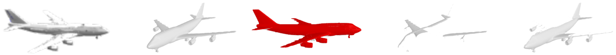
Figure 5.3: To evaluate the reconstruction quality of occluded surfaces, we first align the reconstructed shape (b) with the input image (a) and cast rays onto the surface (c). Next, we identify the (red) faces that intersect with the rays via ray-mesh intersection and separate the reconstructed mesh into (d) visible and (e) occluded areas.
