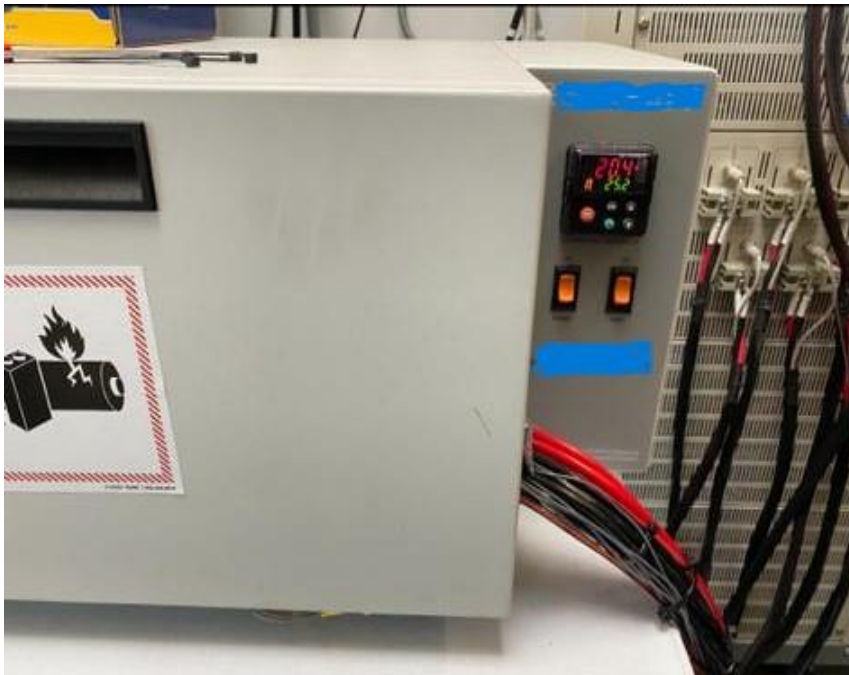
Figure 12. Thermal chamber housing the battery cell.
