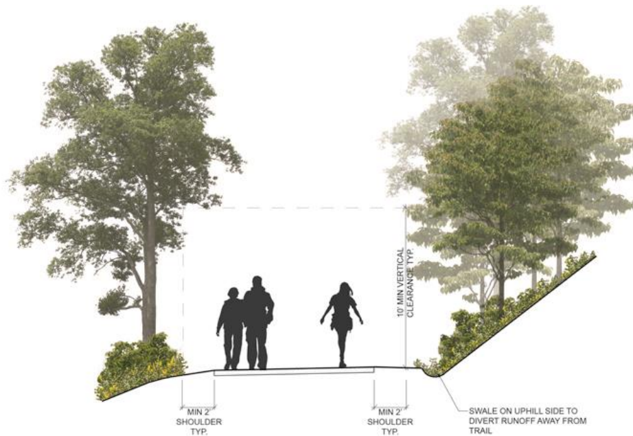
Figure 2-2 Sectional drawing of proposed trail management (Image: Asakura Robinson,)
