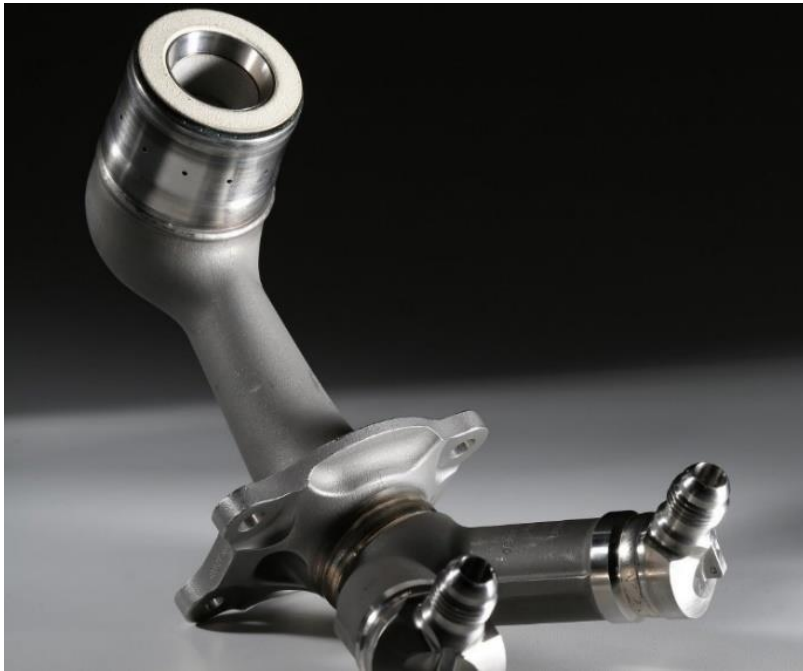
Figure 15. GE LEAP™ Engine Nozzle made by Metal L-PBF Process [5]
