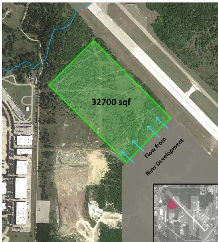
Figure 20 Biofiltration Structure Sizing
