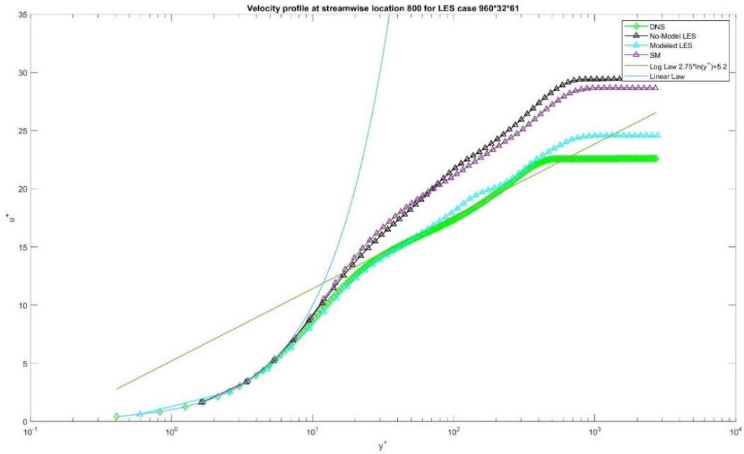
Figure 7. 5 (b) Log profile at streamwise location  $x=800$
