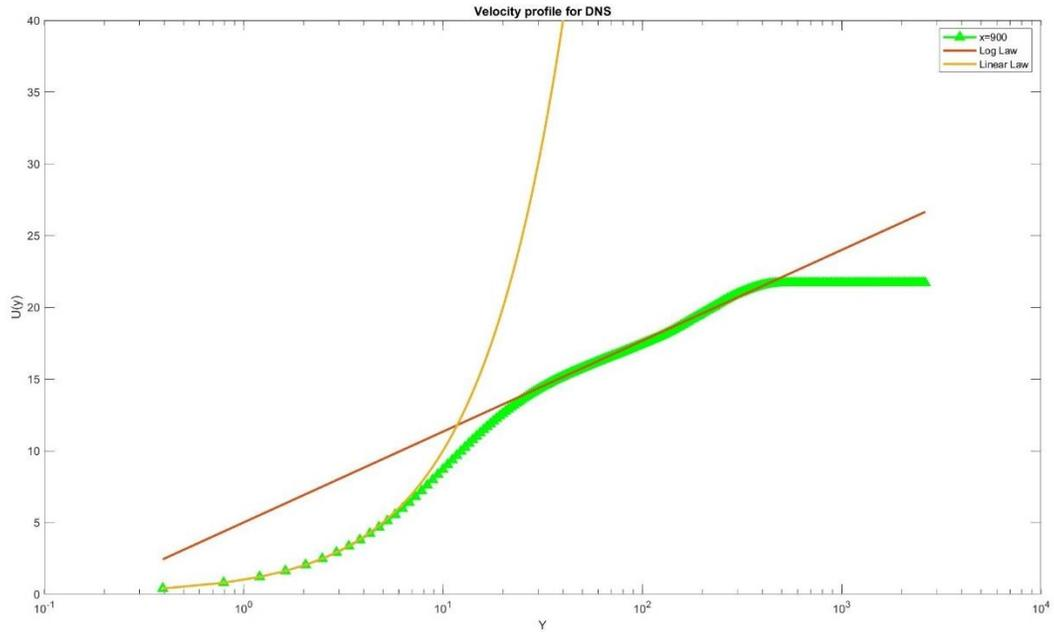
*Figure 7.1 Log profile of DNS flat plate*
