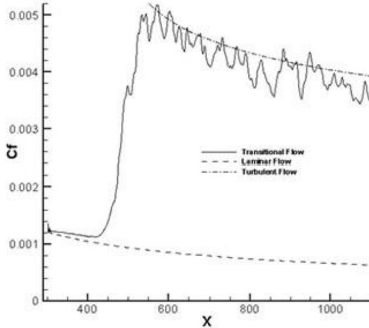
Figure 7.3 Time and spanwise average skin friction coefficient
