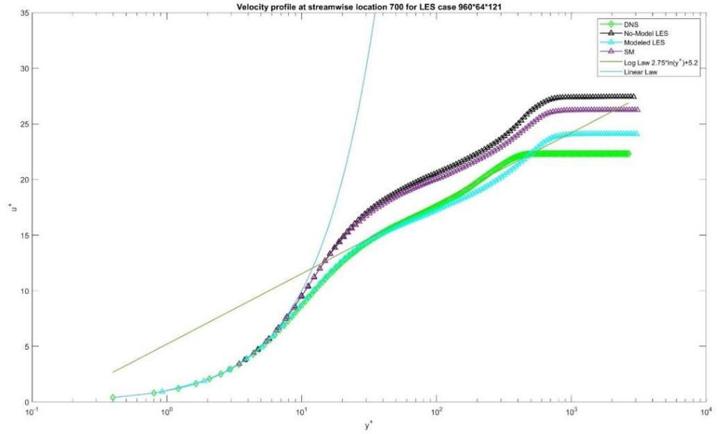
Figure 7.4 (a) Log profile at streamwise location  $x=700$
