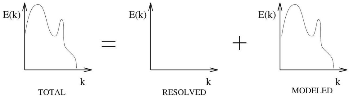
Figure 3.6 Decomposition of the energy spectra of RANS
