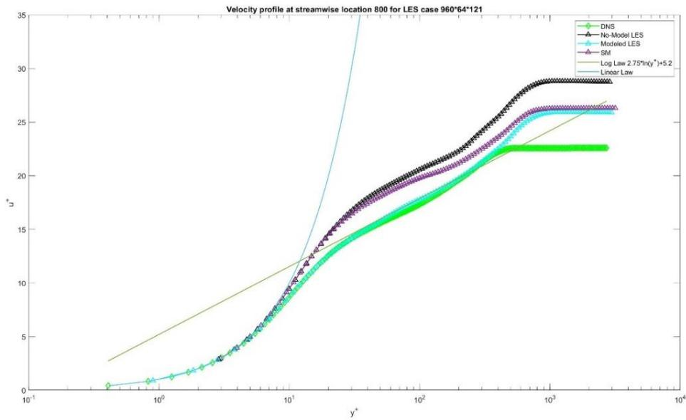
Figure 7.4 (b) Log profile at streamwise location  $x=800$
