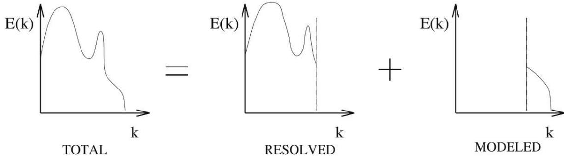
Figure 3.5 Decomposition of energy spectra of LES
