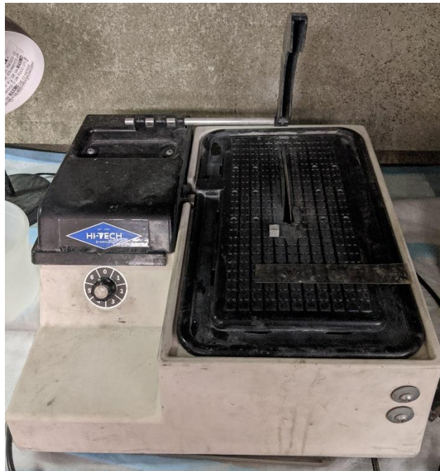
Figure 5: Hi-Tech diamond saw.
