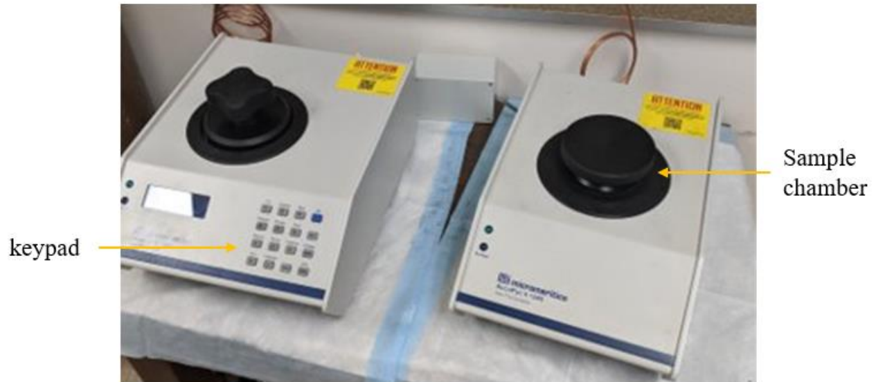
Figure 11: AccuPyc II 1340 control module with keypad on the left and analysis module on the right.
