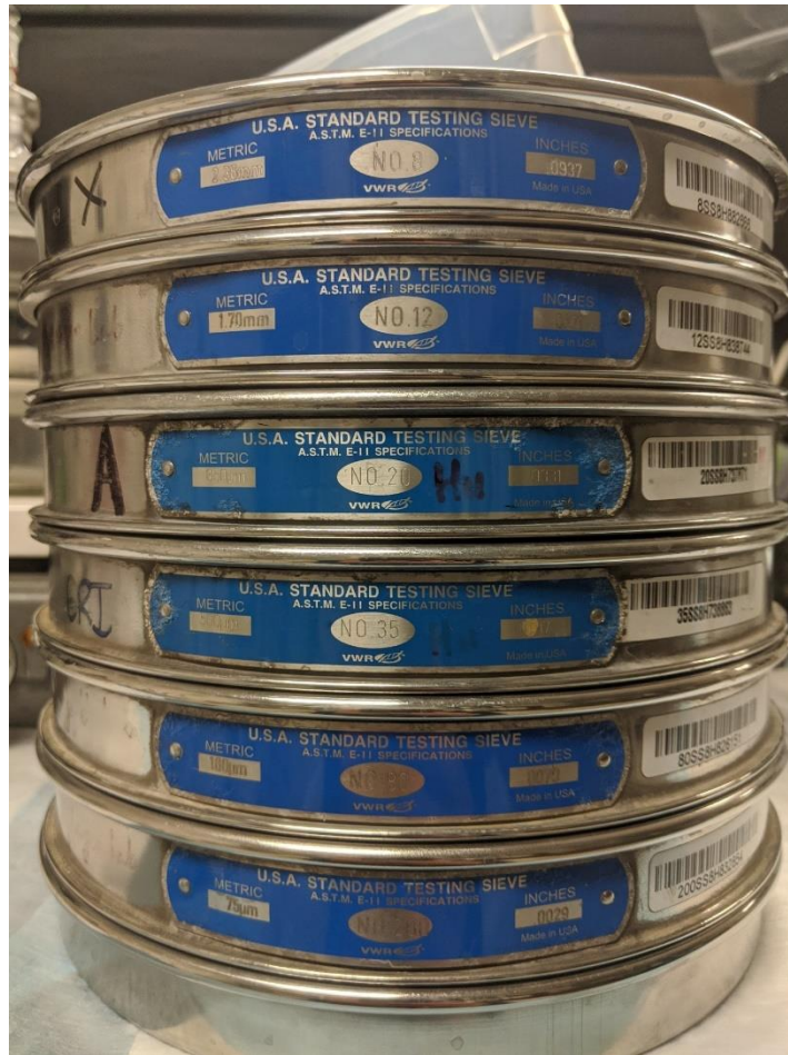
Figure 7: Stacked sieve system.
