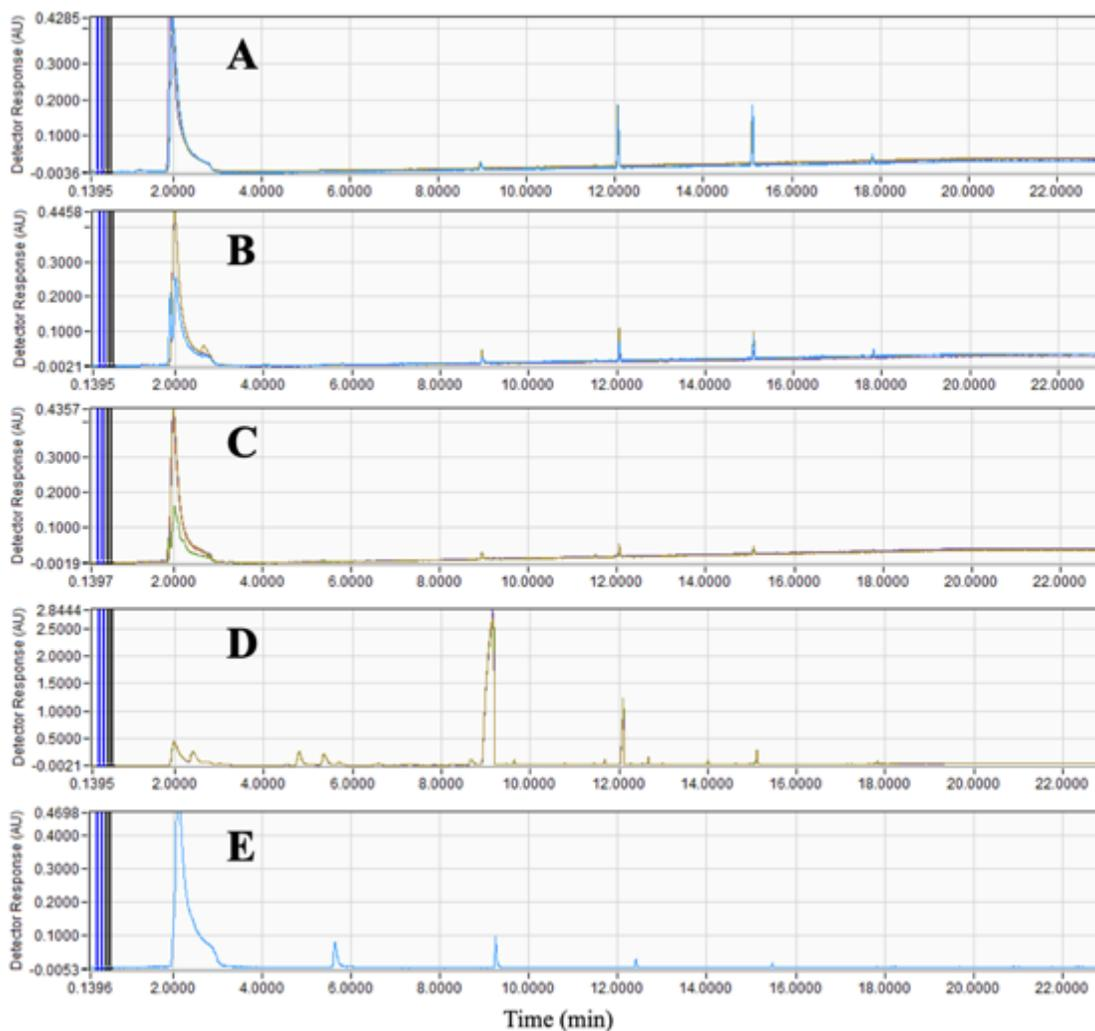
**Figure 3-S7.** Test for outgassing of siloxanes and other contaminants using gas chromatography with a vacuum ultraviolet detector; data is displayed for absorption from 125 – 160 nm. A.) Blank with only air in the vial; B.) Black o-rings; C.) Green o-rings; D.) ThermoGreen® septa; E.) BTO septa.
