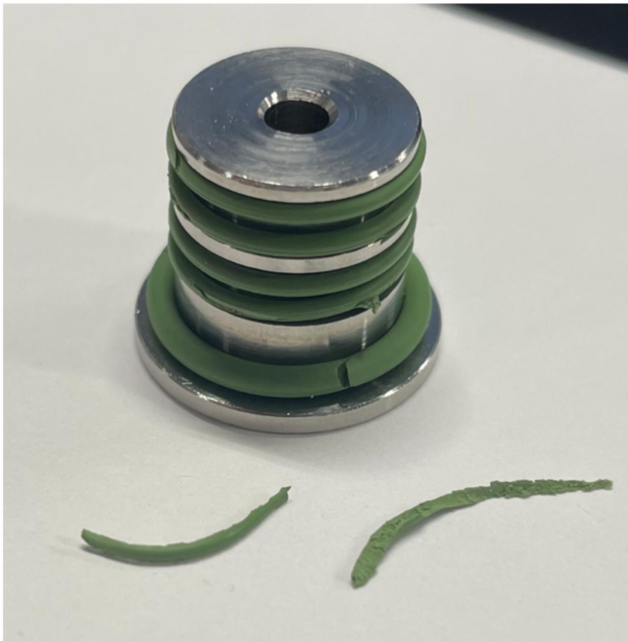
**Figure 3-S6.** Degradation of the green o-rings consisting of hydrogenated nitrile after two to five uses. Pieces of the green o-rings would tear off and eventually rip apart.
