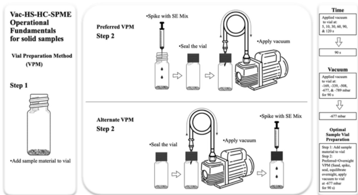
**Figure 3-1.** Vac-HS-HC-SPME operational fundamentals workflow for sample vial preparation of solid samples to be spiked with a standard solution.
