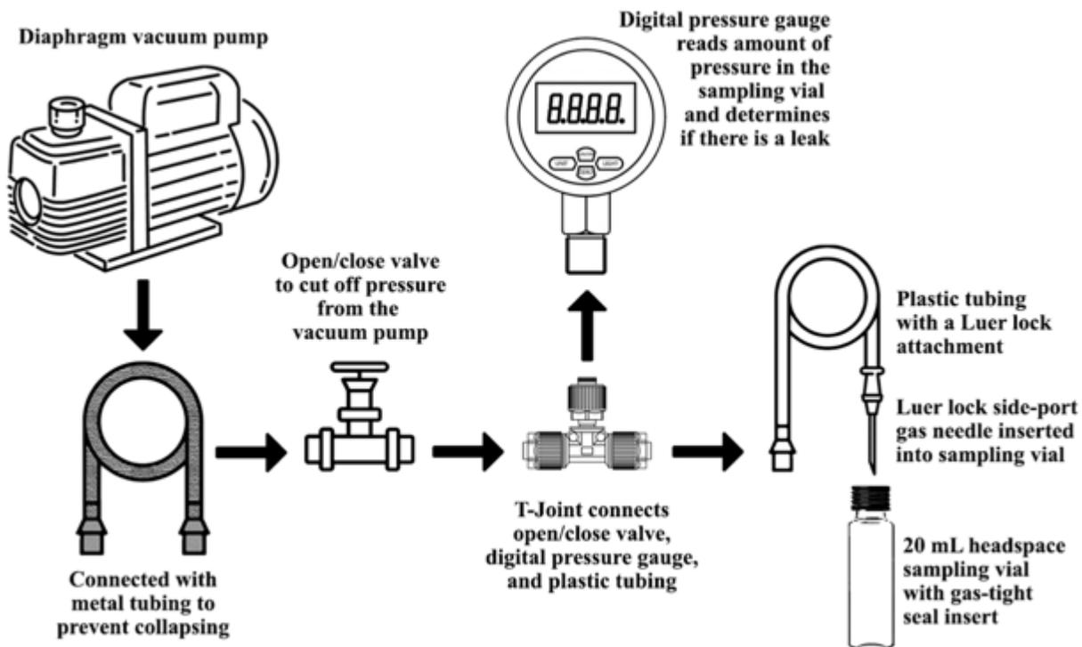
**Figure 2-1.** Vac-HS-SPME sampling setup
