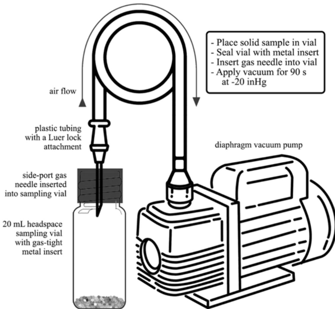
**Figure 4-2.** Vac-HS-HC-SPME Sampling Setup
