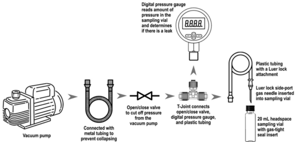
**Figure 3-5.** Apparatus for applying vacuum to headspace vials.
