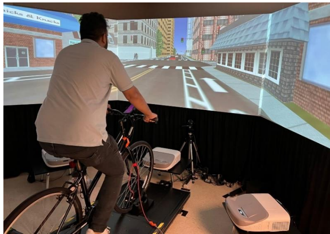
Figure 1: Bike simulator setup at UTA Human Factors lab
