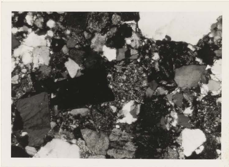
Fig. 1. Chert cement filling the spaces between rock fragments.
