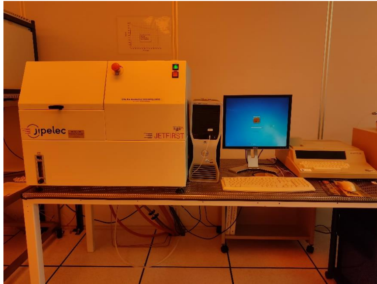
Figure 19: JetFirst Rapid Thermal Annealing for Heating samples
