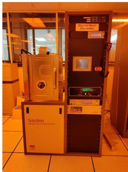
Figure 21: CHA E-Beam Solution for metal deposition
