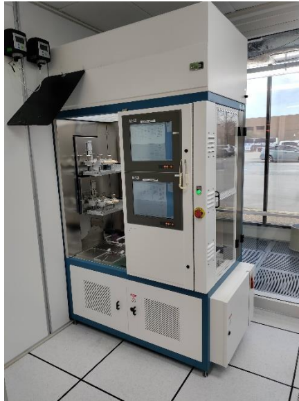
Figure 5: Tystar Oxidation Furnace for Thermal Oxidation and nitride of Silicon
