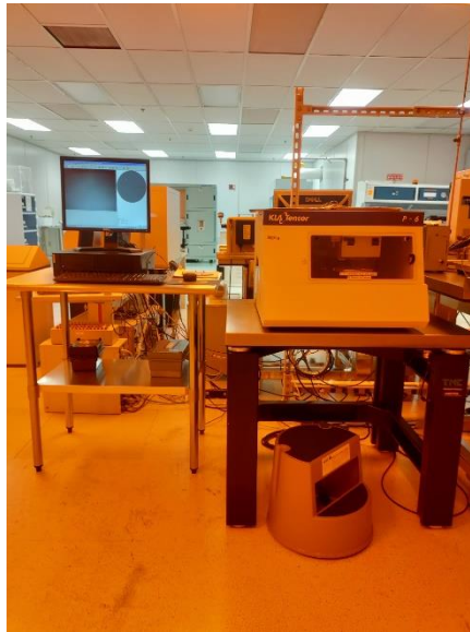
Figure 10: KLA Tencor-P6 profilometer for profile measurement
