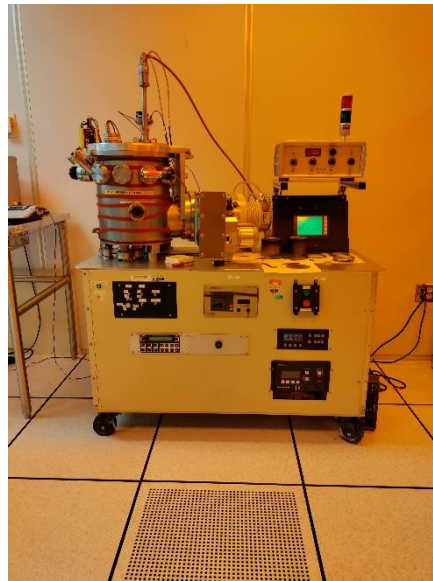
Figure 13: Homebuilt Sputter deposition equipment for DC and RF Sputter deposition
