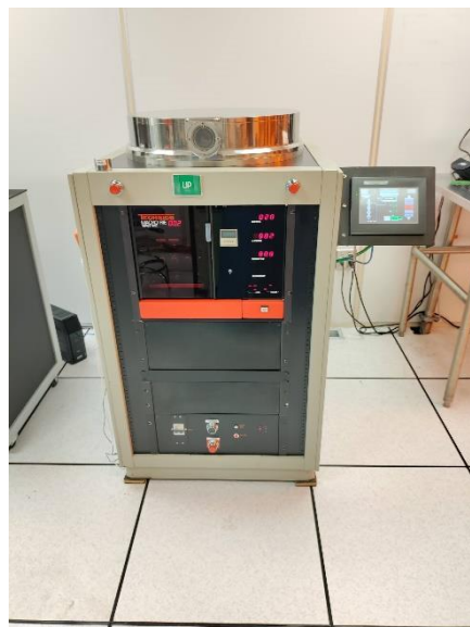
Figure 9: Technics Macro RIE – 8800 equipment for Reactive Ion Etching
