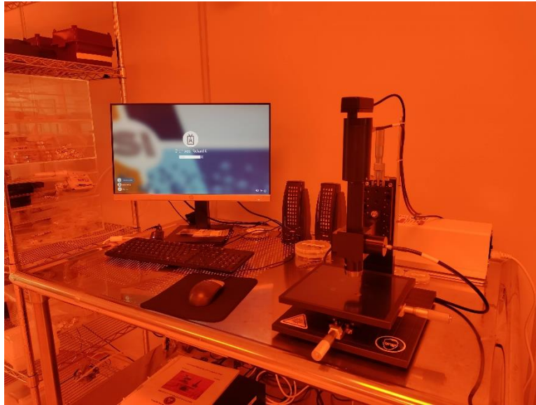
Figure 20: Ocean Optics Reflectometer for thickness measurement
