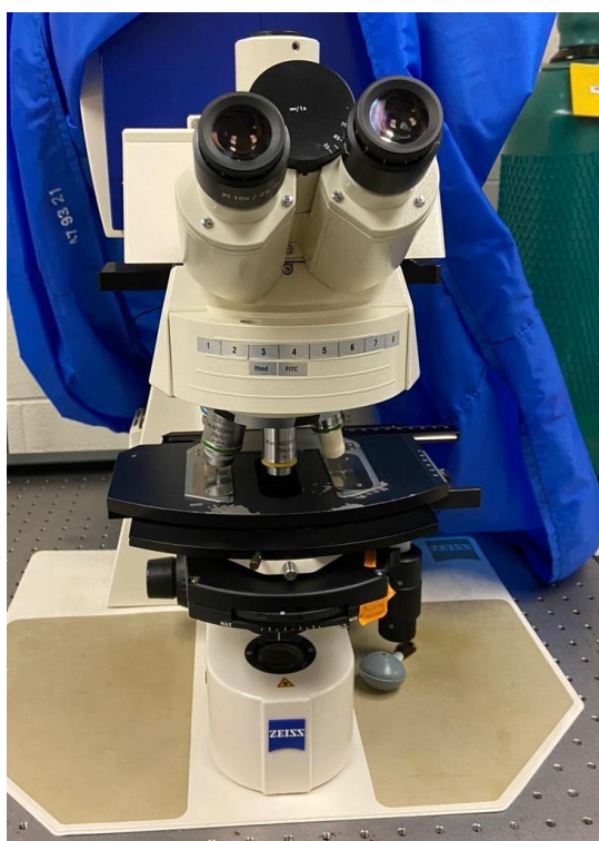
Figure 3.1.1 Zeiss Axioscope 5 Optical Microscope
